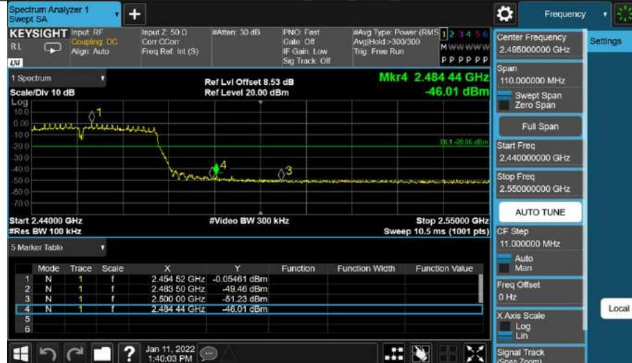
Note: 1. Testing was carried out within frequency range 9kHz to the tenth harmonics. The measurement results below 30MHz and 18GHz - 26.5GHz were greater than 20dB below the limit, so only the radiated spurious emissions from 30MHz to 18GHz were reported. 2. This testing was carried out on different modulations, but only the worst case was presented in this report. 3. We tested four adapter and recorded the wose case data in the report.
