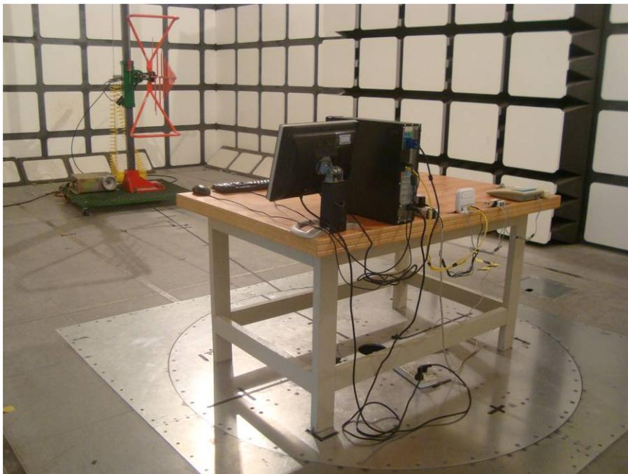
**Radiated Emissions - Front View (Model: ZXDSL 831 II with adapter 2)**
