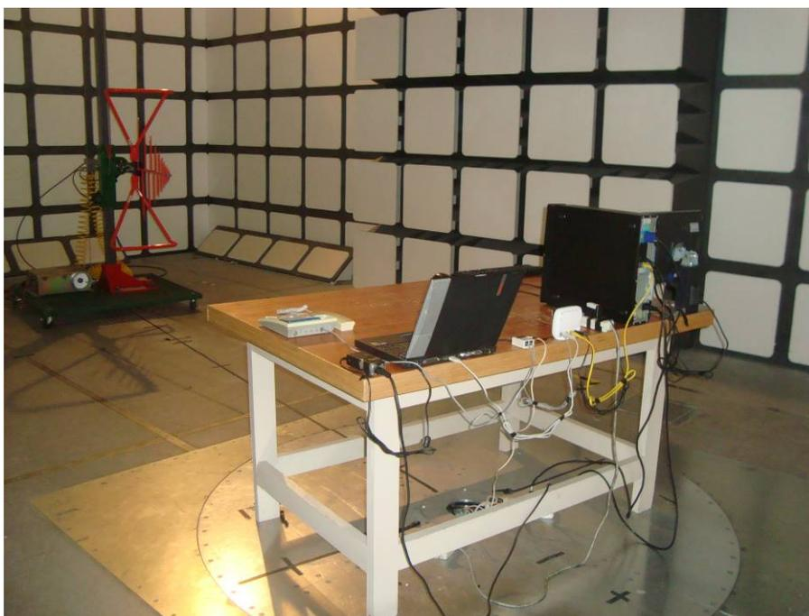
**Radiated Emissions - Front View (Model: ZXDSL 831A II with adapter 2)**
