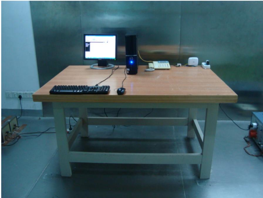
**Conduction Emissions - Side View (Model: ZXDSL 831 II with adapter 1)**
