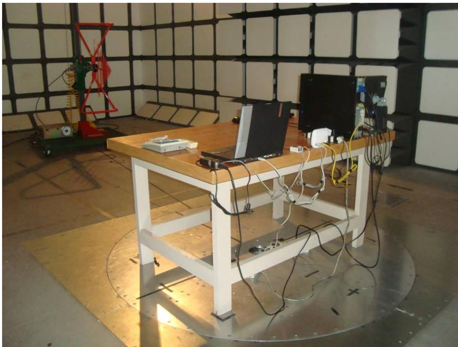
**Radiated Emissions - Front View (Model: ZXDSL 831 II with adapter 1)**
