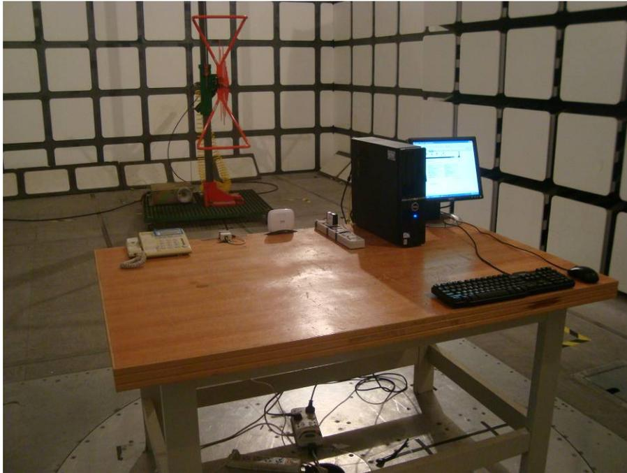
**Radiated Emissions - Rear View (Model: ZXDSL 831 II with adapter 2)**
