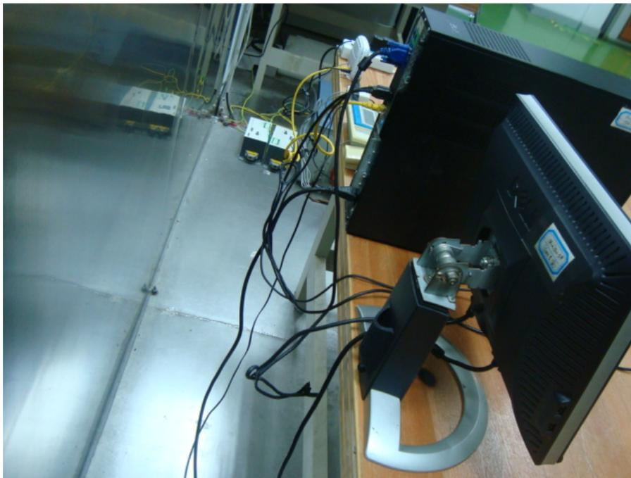
**Radiated Emissions - Front View (Model: ZXDSL 831A II with adapter 1)**
