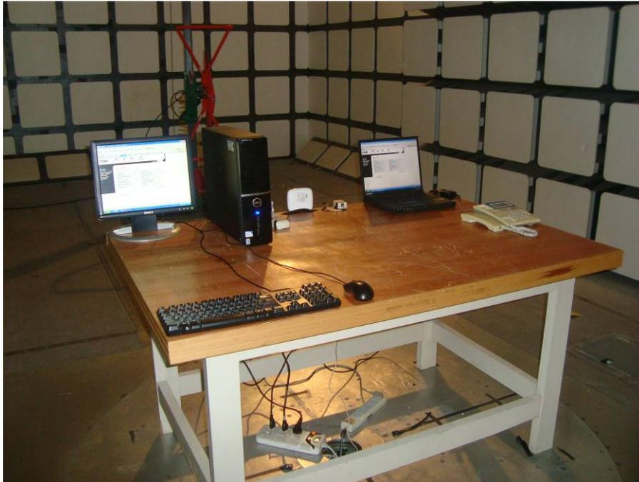
**Radiated Emissions - Rear View (Model: ZXDSL 831A II with adapter 2)**
