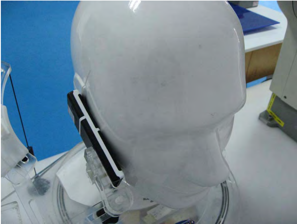
Fig.5 EUT Right Head Touch Cheek Position
