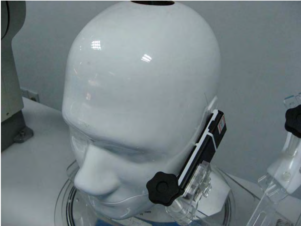
Fig.3 EUT Left Head Touch Cheek Position
