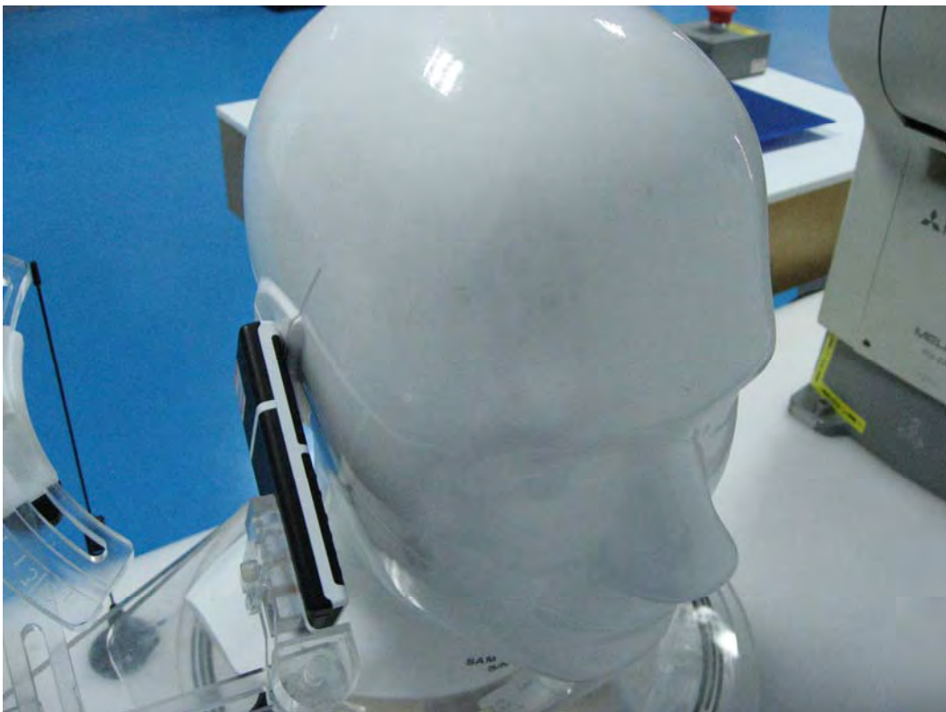
Fig.6 EUT Right Head Tilt15 Position
