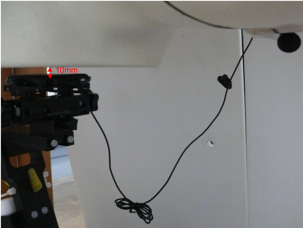
Picture 19: Back Side with earphone, the distance from handset to the bottom of the Phantom is 10mm
