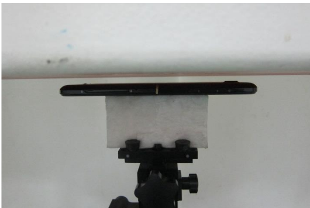
Bottom Face of Tablet with Phantom 0.8 cm Gap
