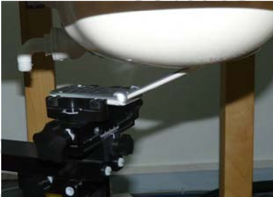
Picture 4 Head SAR tilt position
