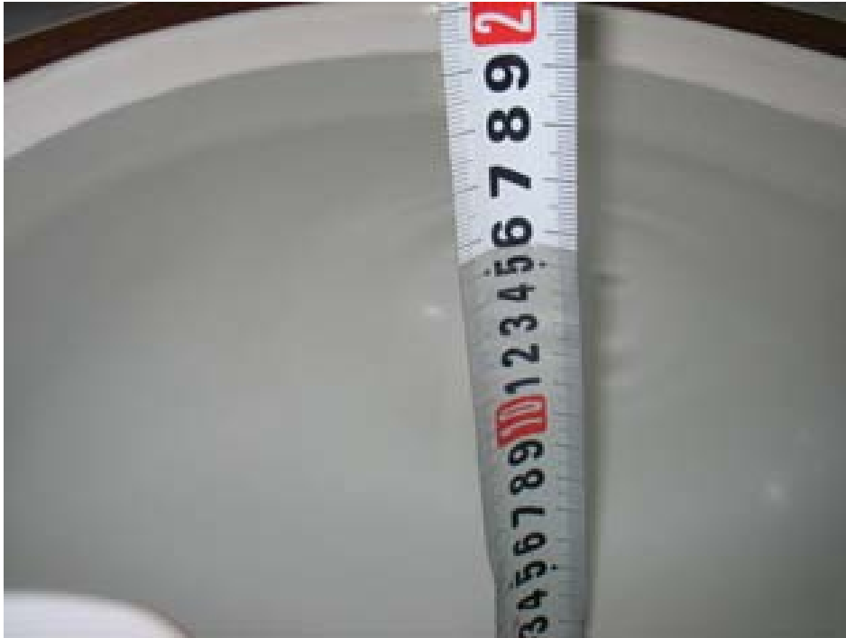
Picture 9 Liquid Depth at Ear Reference Point for 1900MHz Head Liquid
