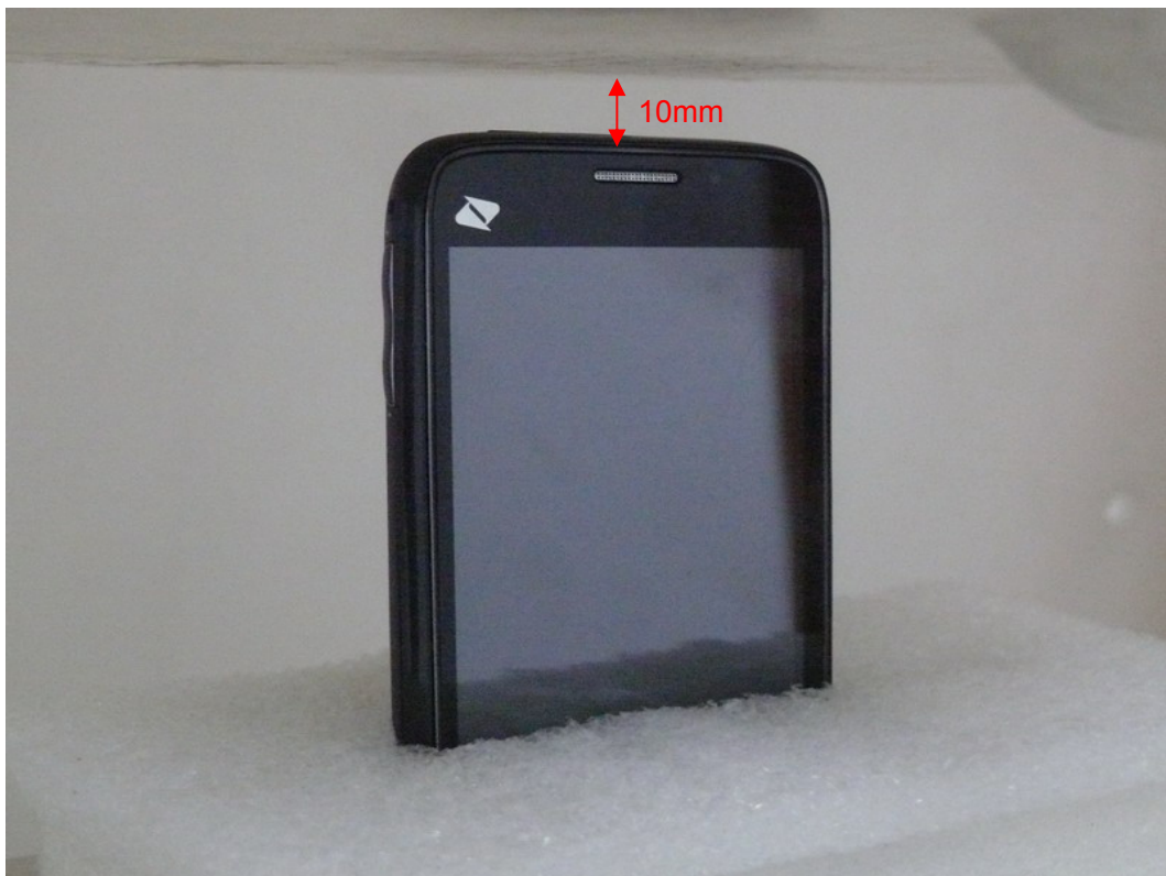
Picture 18: Top edge, the distance from handset to the bottom of the Phantom is 10mm
