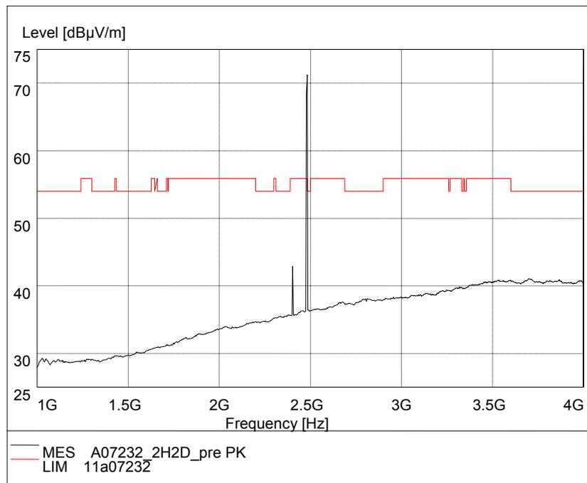
Fig.77. Radiated emission:  $\pi/4$  DQPSK, Channel 78, 1 GHz - 4 GHz
