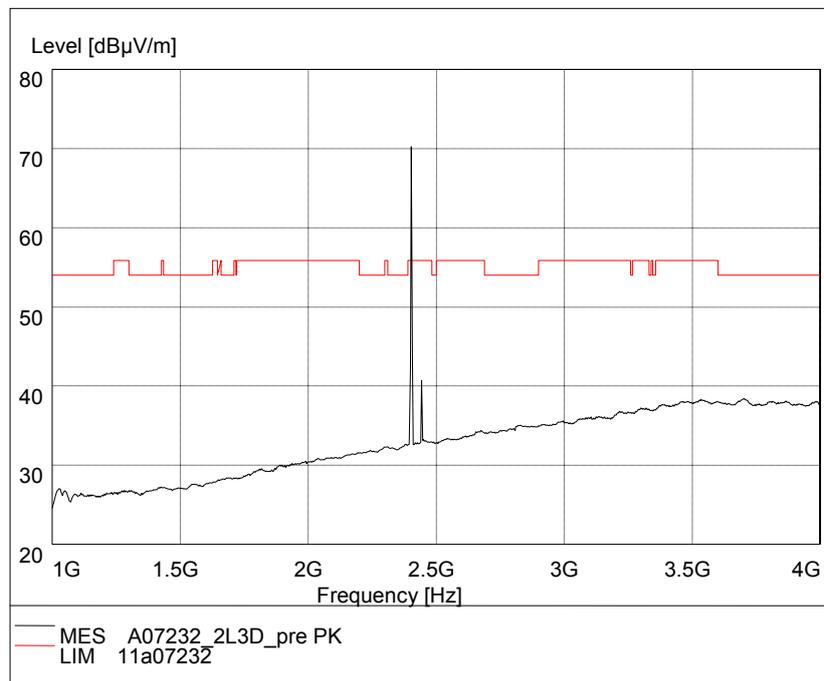
Fig.83. Radiated emission: 8DPSK, Channel 0, 1 GHz - 4 GHz
