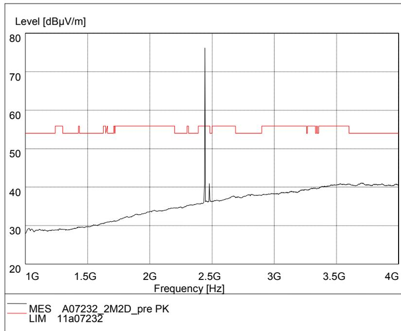
Fig.74. Radiated emission:  $\pi/4$  DQPSK, Channel 39, 1 GHz - 4 GHz
