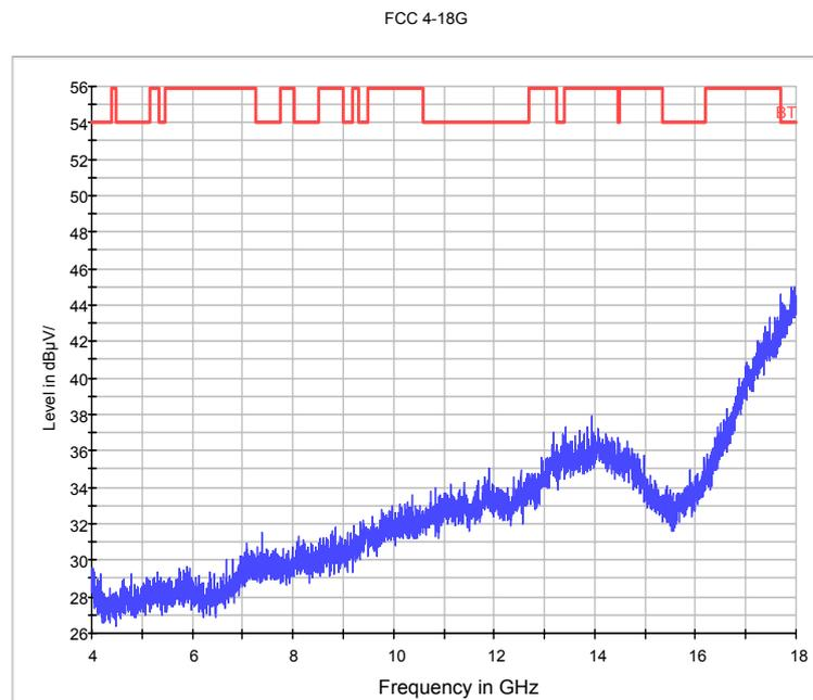
Fig.63. Radiated emission: GFSK, Channel 39, 4 GHz - 18 GHz
