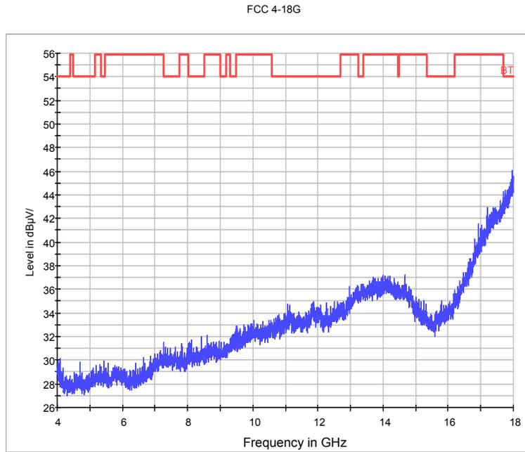
Fig.66. Radiated emission: GFSK, Channel 78, 4 GHz - 18 GHz
