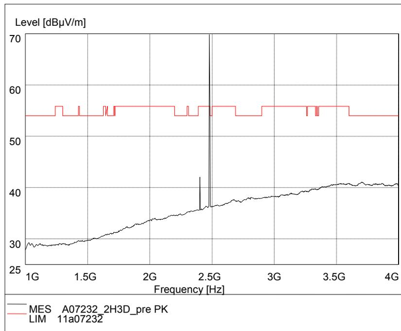
Fig.89. Radiated emission: 8DPSK, Channel 78, 1 GHz - 4 GHz
