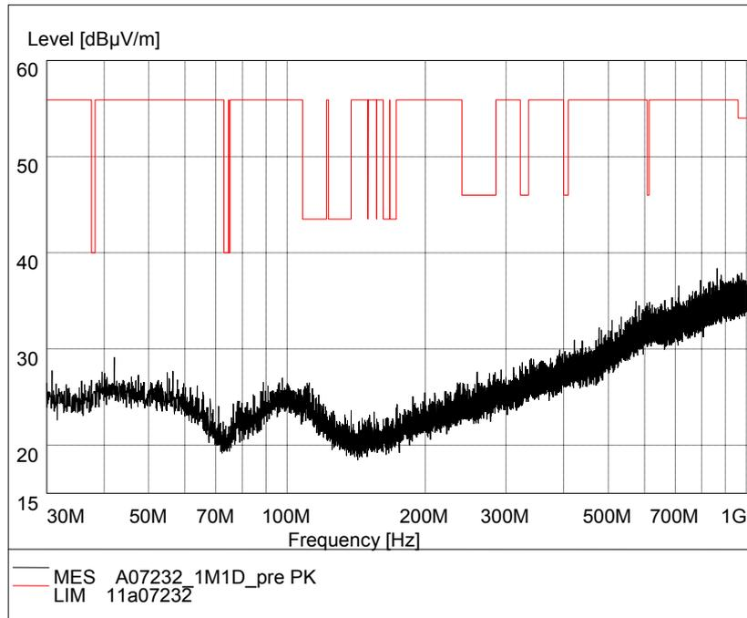
Fig.61. Radiated emission: GFSK, Channel 39, 30 MHz - 1 GHz
