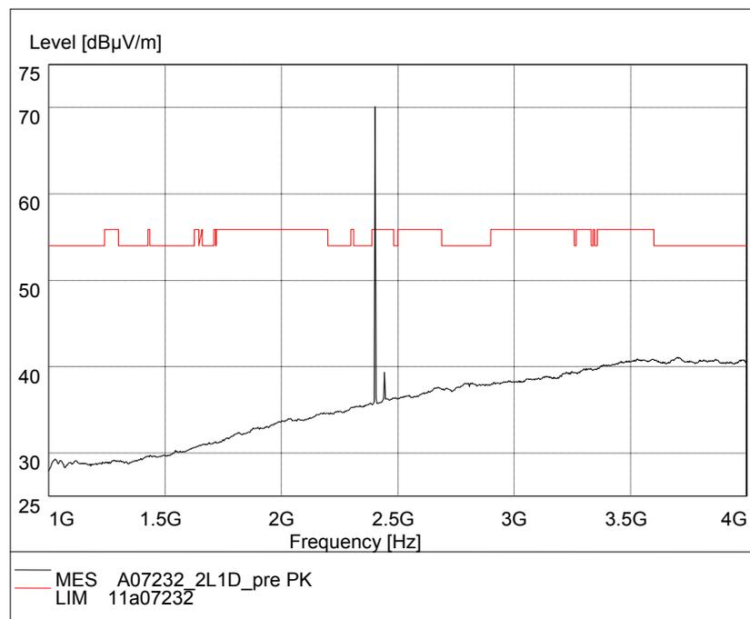
Fig.59. Radiated emission: GFSK, Channel 0, 1 GHz - 4 GHz
