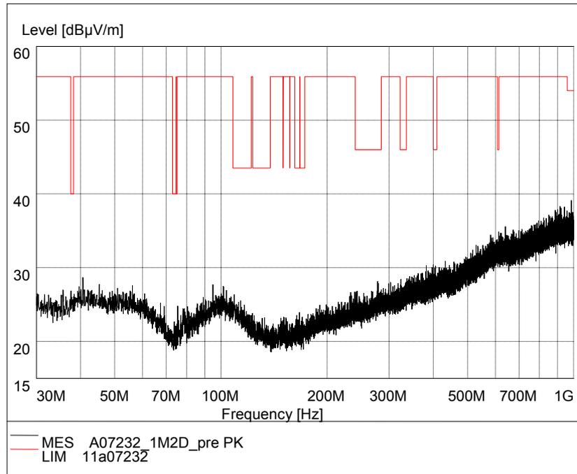
Fig.73. Radiated emission:  $\pi/4$  DQPSK, Channel 39, 30 MHz - 1 GHz
