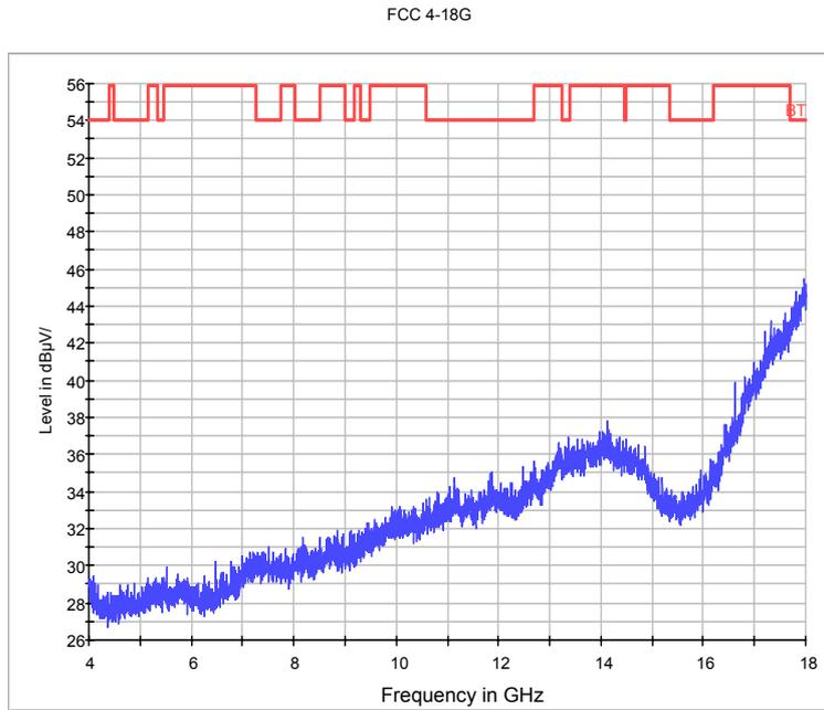
Fig.60. Radiated emission: GFSK, Channel 0, 4 GHz - 18 GHz
