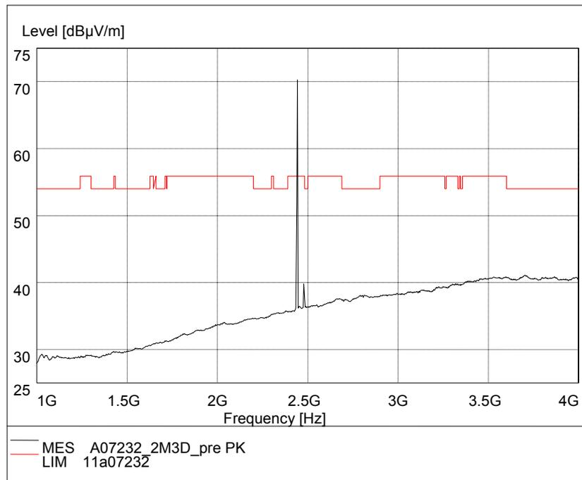
Fig.86. Radiated emission: 8DPSK, Channel 39, 1 GHz - 4 GHz
