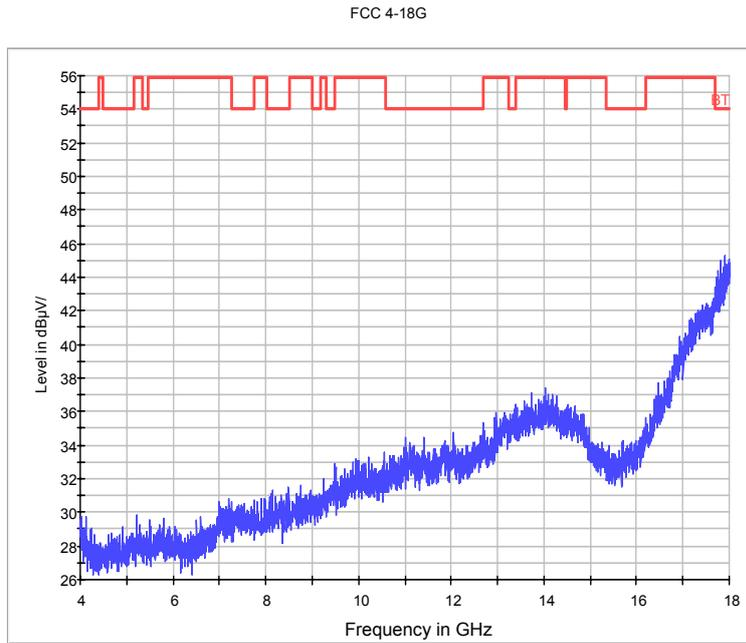
Fig.84. Radiated emission: 8DPSK, Channel 0, 4 GHz - 18 GHz
