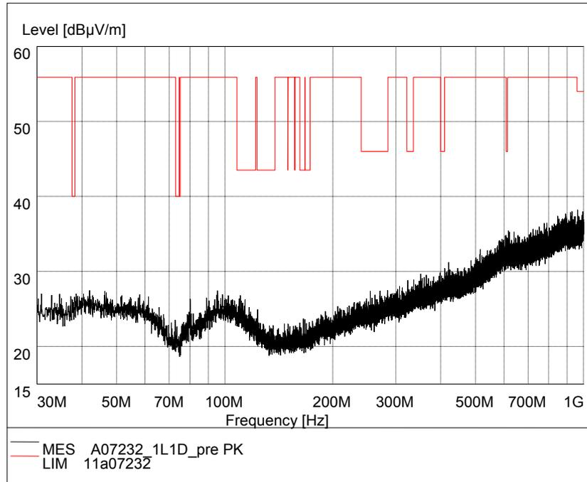
Fig.58. Radiated emission: GFSK, Channel 0, 30 MHz - 1 GHz
