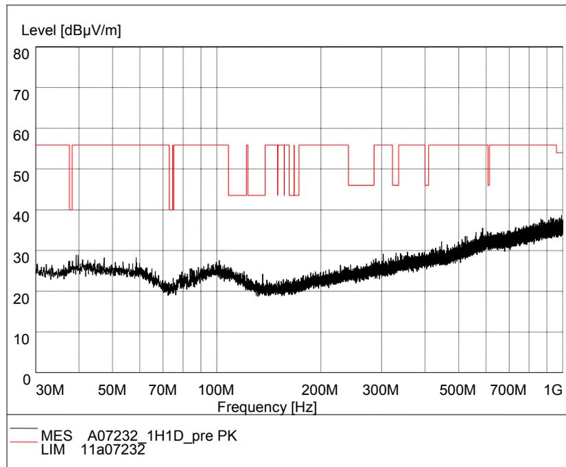
Fig.64. Radiated emission: GFSK, Channel 78, 30 MHz - 1 GHz
