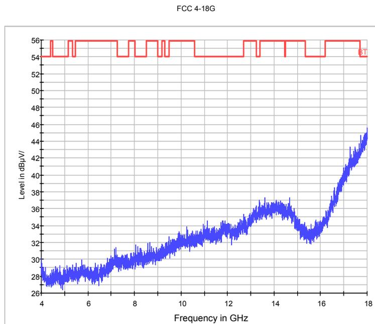
Fig.87. Radiated emission: 8DPSK, Channel 39, 4 GHz - 18 GHz
