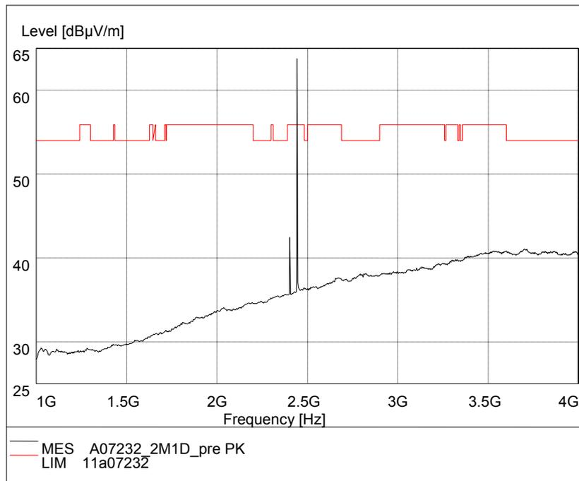
Fig.62. Radiated emission: GFSK, Channel 39, 1 GHz - 4 GHz
