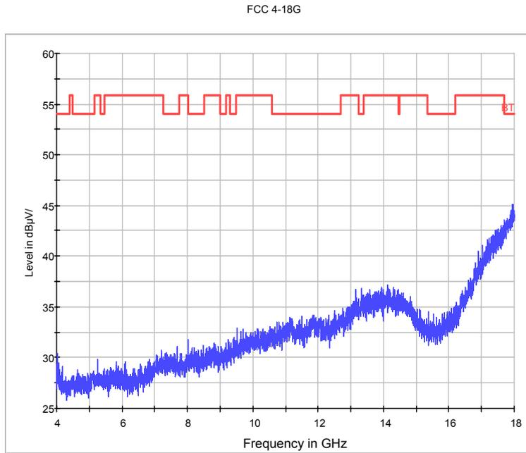
Fig.78. Radiated emission:  $\pi/4$  DQPSK, Channel 78, 4 GHz - 18 GHz
