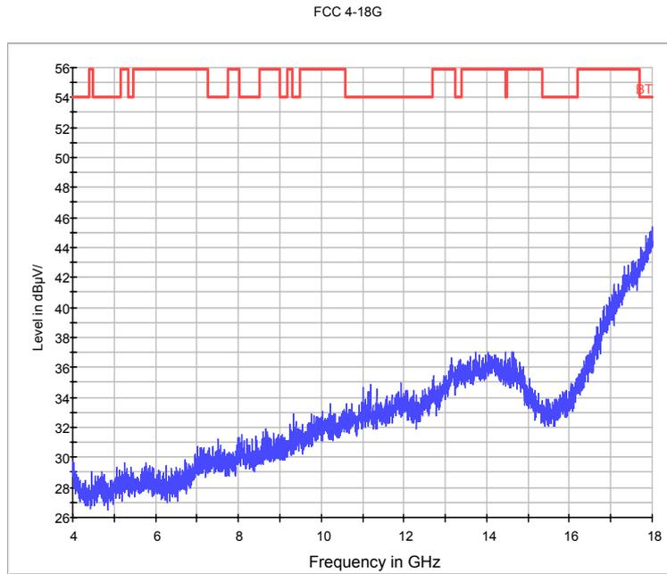
Fig.90. Radiated emission: 8DPSK, Channel 78, 4 GHz - 18 GHz
