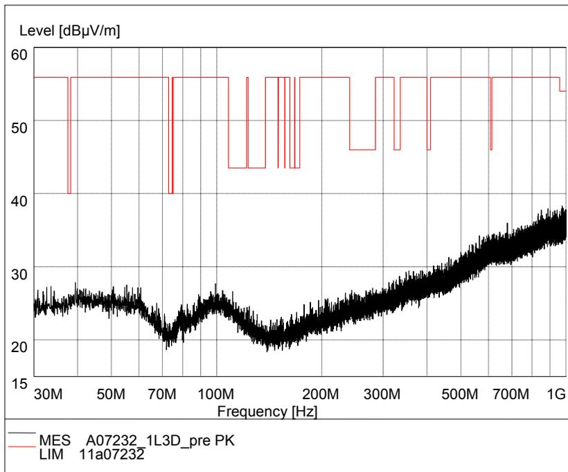
Fig.82. Radiated emission: 8DPSK, Channel 0, 30 MHz - 1 GHz
