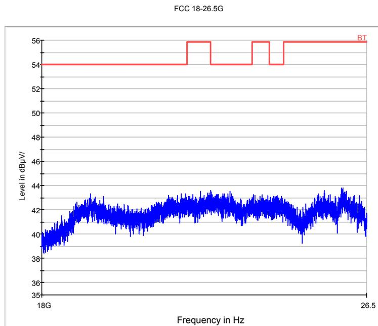
Fig.69. Radiated emission: GFSK, 18 GHz - 26 GHz
