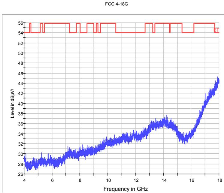
Fig.72. Radiated emission:  $\pi/4$  DQPSK, Channel 0, 4 GHz - 18 GHz
