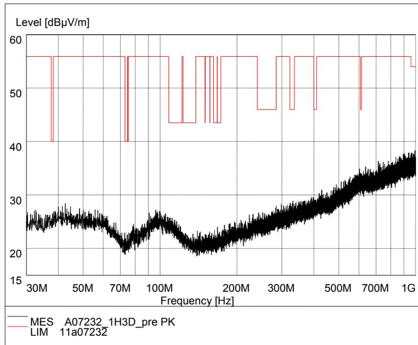
Fig.88. Radiated emission: 8DPSK, Channel 78, 30 MHz - 1 GHz
