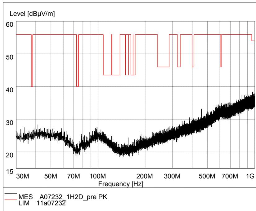
Fig.76. Radiated emission:  $\pi/4$  DQPSK, Channel 78, 30 MHz - 1 GHz
