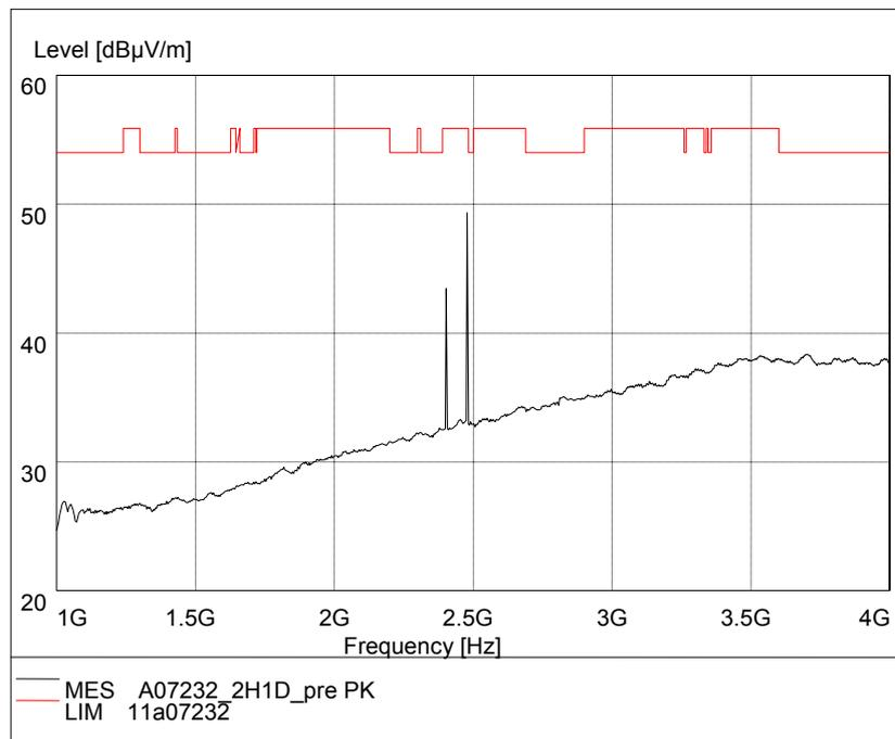
Fig.65. Fig.47 Radiated emission: GFSK, Channel 78, 1 GHz - 4 GHz
