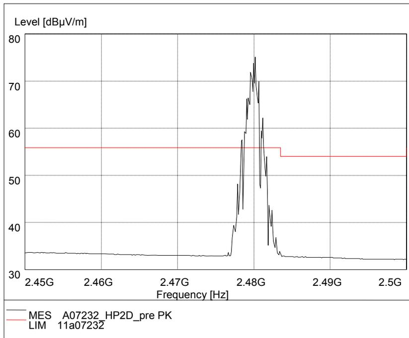
Fig.80. Radiated emission (Power):  $\pi/4$  DQPSK, high channel
