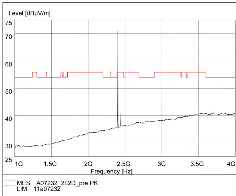
Fig.71. Radiated emission:  $\pi/4$  DQPSK, Channel 0, 1 GHz - 4 GHz
