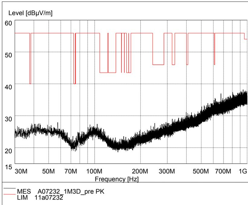
Fig.85. Radiated emission: 8DPSK, Channel 39, 30 MHz - 1 GHz
