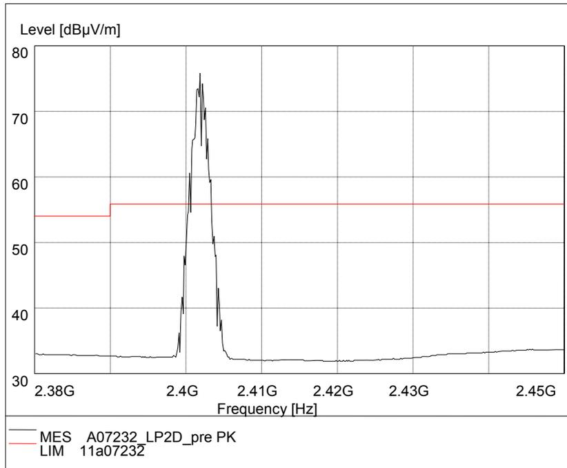
Fig.79. Radiated emission (Power):  $\pi/4$  DQPSK, low channel
