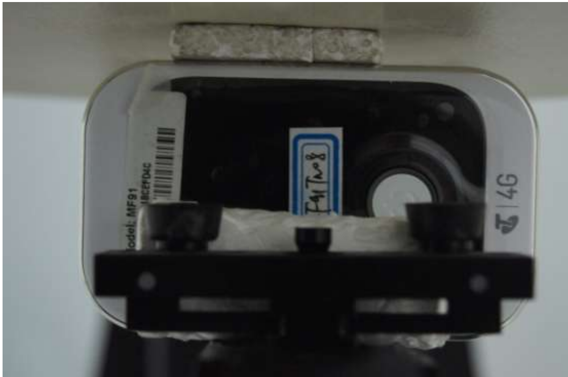
POSITION OF RIGHT SIDE with 10mm distance
