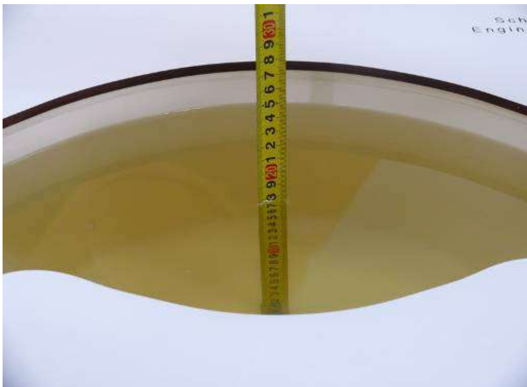
Picture 2: Liquid depth in the flat Phantom (835MHz) (17.5cm deep)
