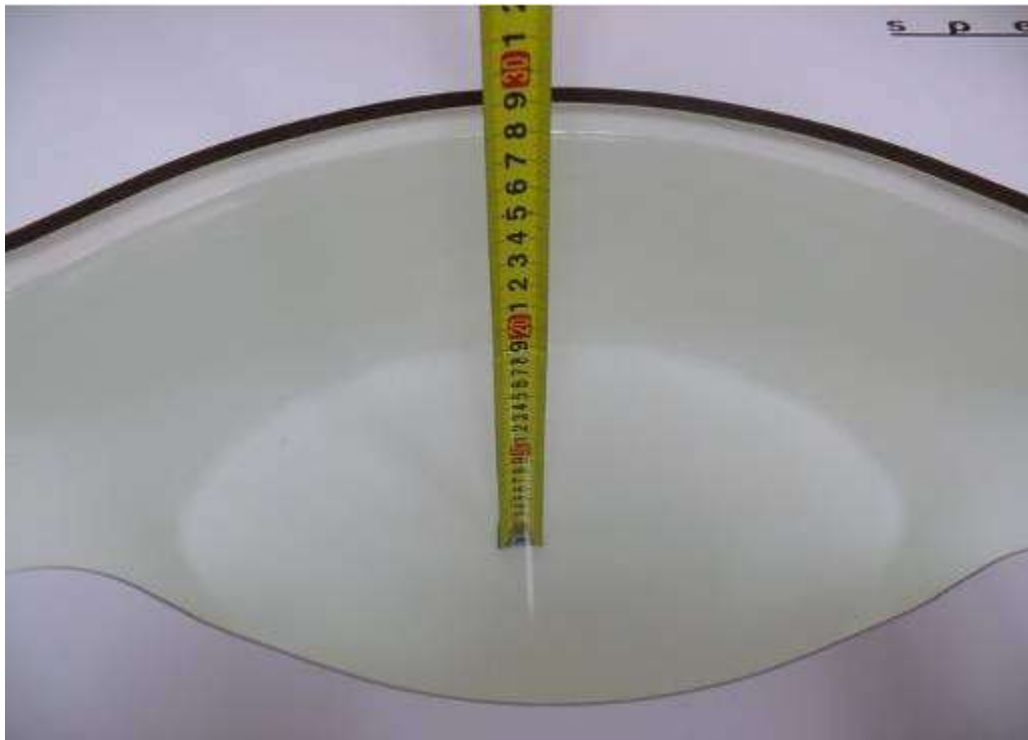
Picture 4: Liquid depth in the flat Phantom (1900 MHz) (19cm deep)
