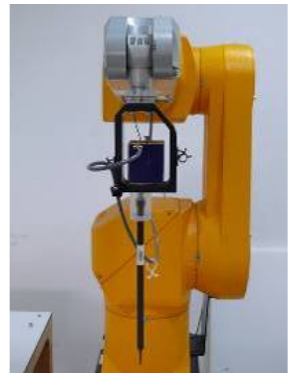
Figure 3. EX3DV4 E-field probe
