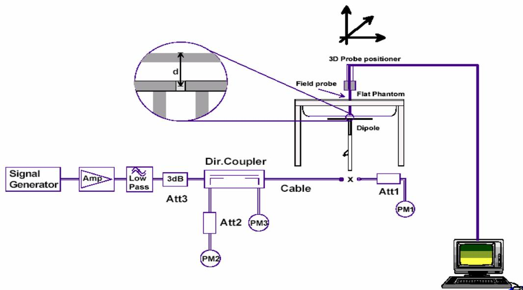
**Fig6. Setup for system performance Check**
