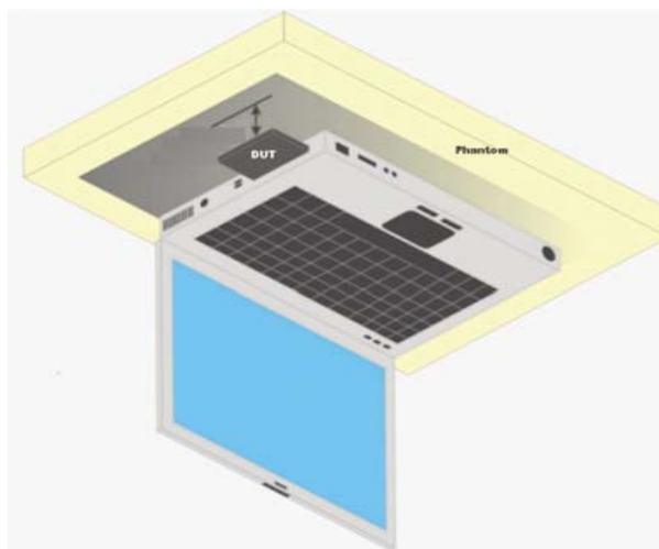
Fig. 3 Lap-held position, bottom of the computer is touching the phantom
