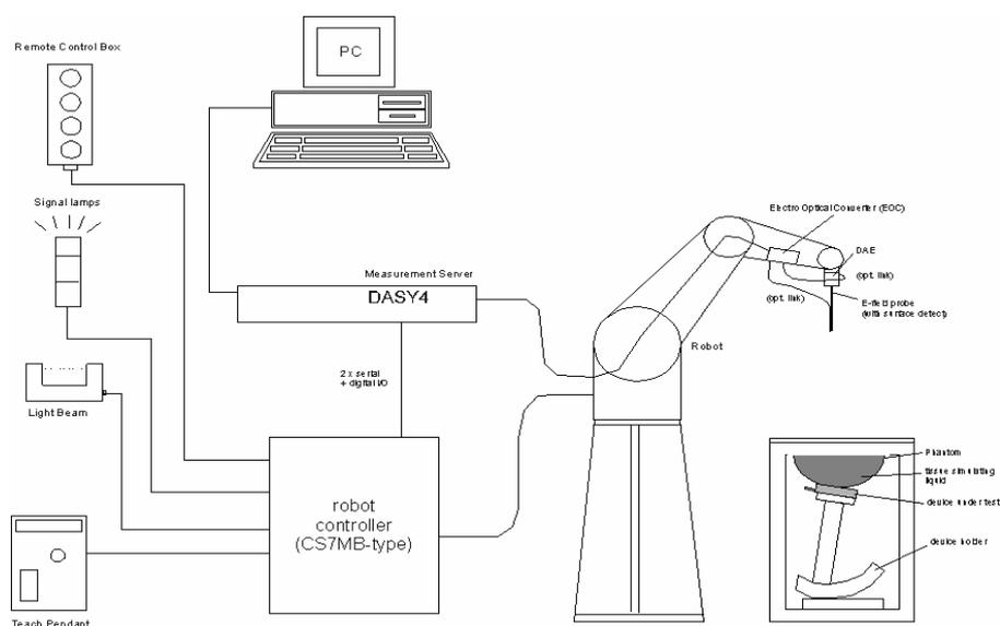
Fig4. The DASY5 measurement system
