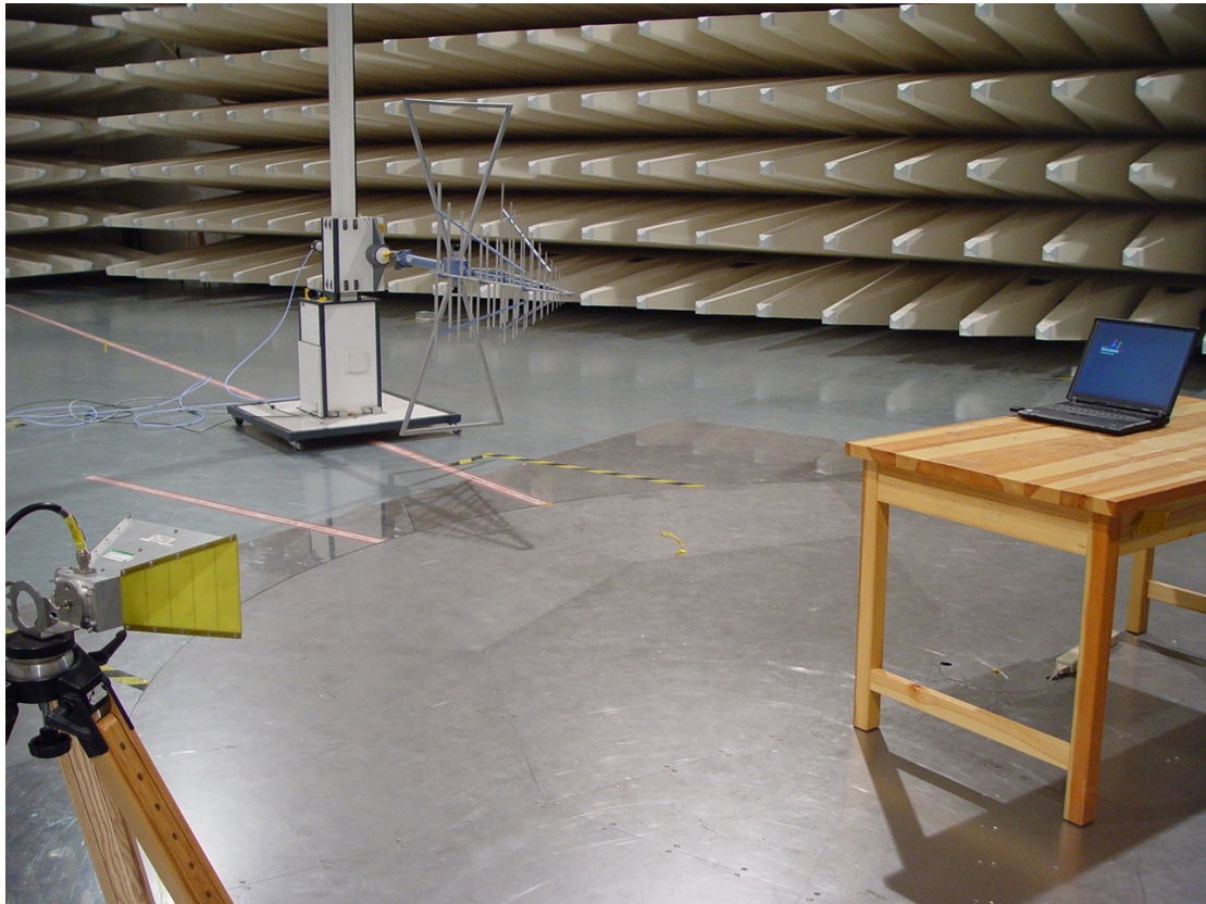
Pic 1 Radiated Emissions Test Setup
