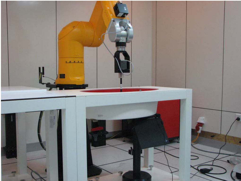
Fig 5. The measurement set-up with ELI 4.0 phantom containing tissue simulating liquid.
