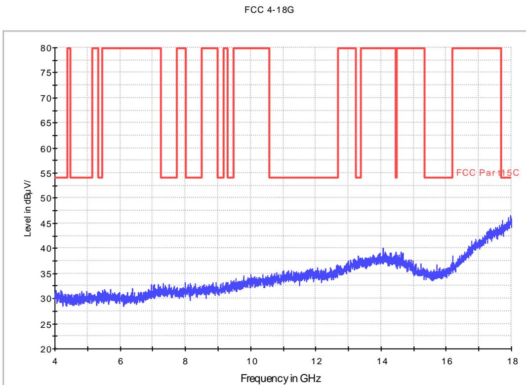
**Fig. 50 Radiated Spurious Emission (802.11g, Ch11, 4 GHz-18 GHz)**
