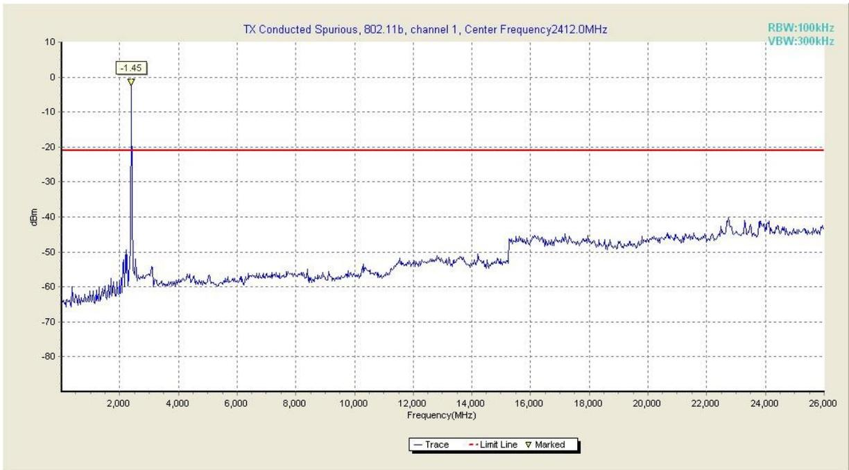
**Fig. 18 Conducted Spurious Emission (802.11b, Ch1, 30 MHz-26 GHz)**
