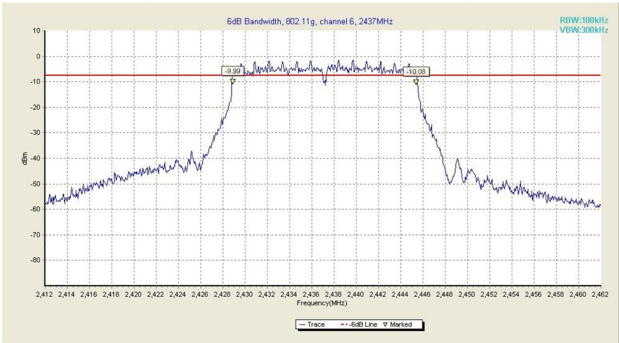
**Fig. 11 Occupied 6dB Bandwidth (802.11g, Ch 6)**
