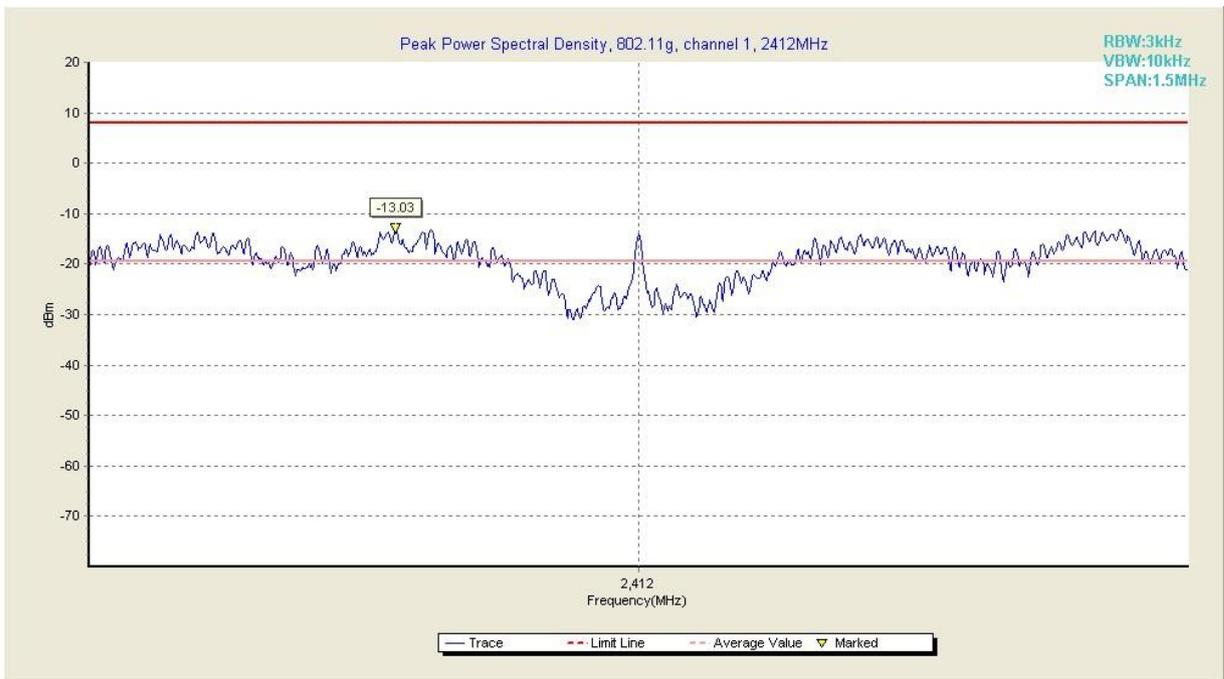
**Fig. 4 Power Spectral Density (802.11g, Ch 1)**
