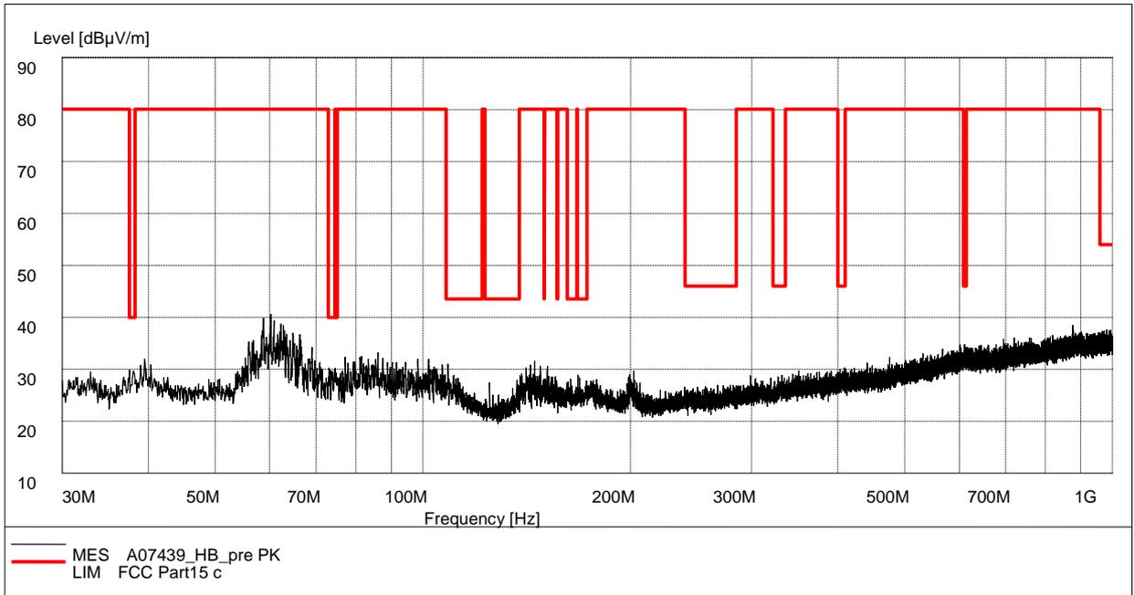
**Fig. 37 Radiated Spurious Emission (802.11b, Ch11, 30 MHz-1 GHz)**
