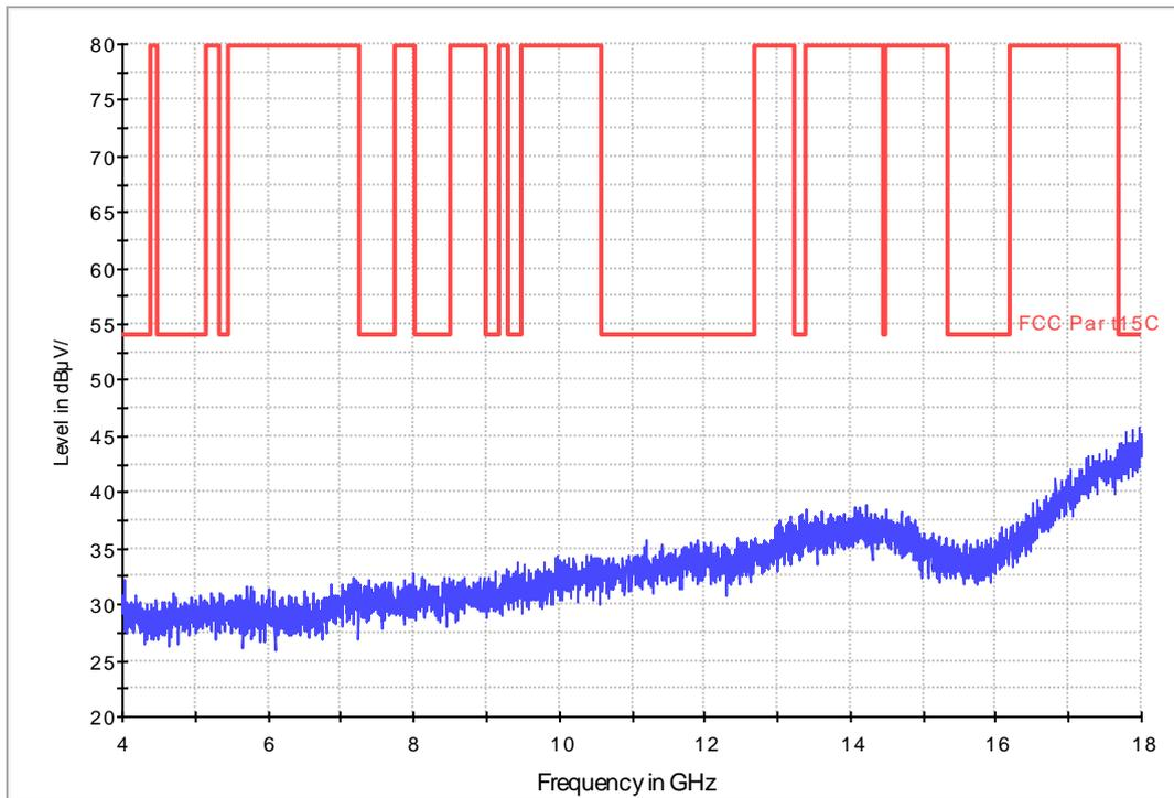
**Fig. 39 Radiated Spurious Emission (802.11b, Ch11, 4 GHz-18 GHz)**
