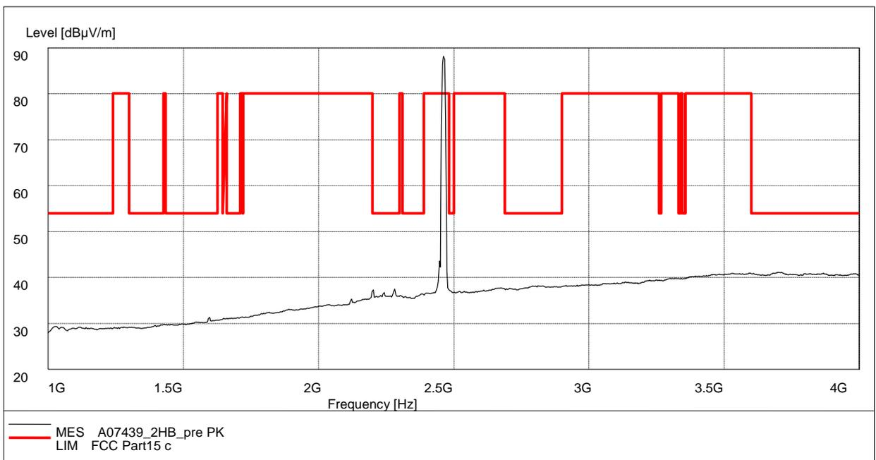
**Fig. 38 Radiated Spurious Emission (802.11b, Ch11, 1 GHz-4 GHz)**
