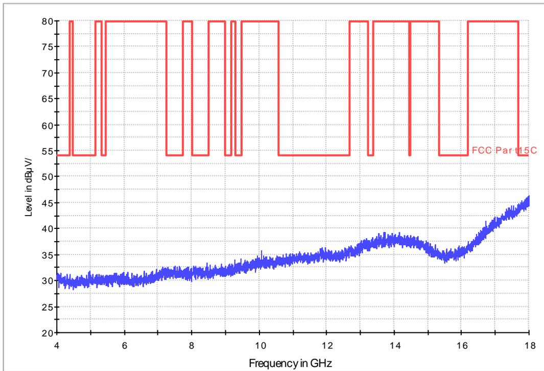
Fig. 43 Radiated Spurious Emission (802.11g, Ch1, 4 GHz-18 GHz)
