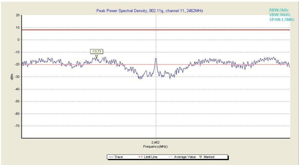
**Fig. 6 Power Spectral Density (802.11g, Ch 11)**
