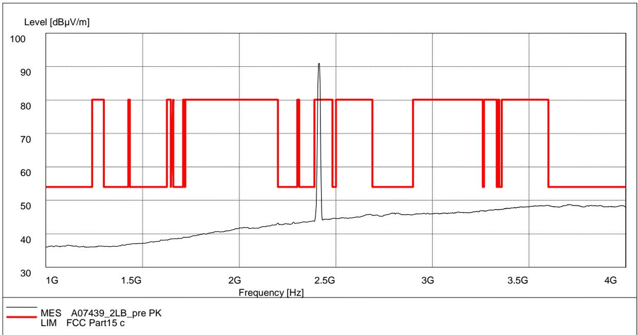
**Fig. 31 Radiated Spurious Emission (802.11b, Ch1, 1 GHz-4 GHz)**
