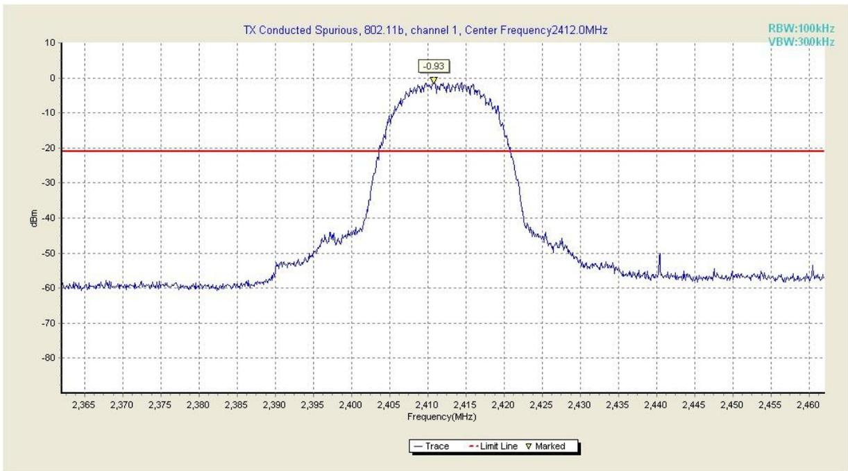
**Fig. 17 Conducted Spurious Emission (802.11b, Ch1, Center Frequency)**
