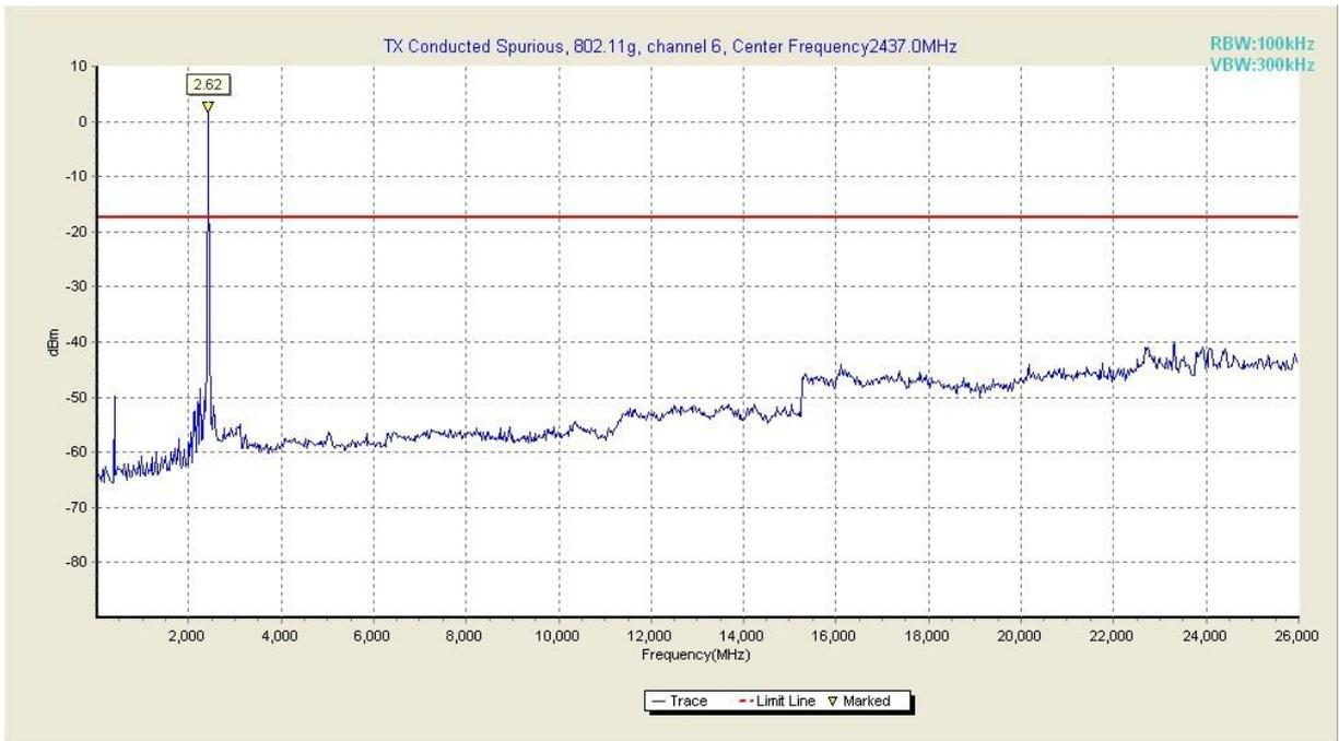
**Fig. 26 Conducted Spurious Emission (802.11g, Ch6, 30 MHz-26 GHz)**
