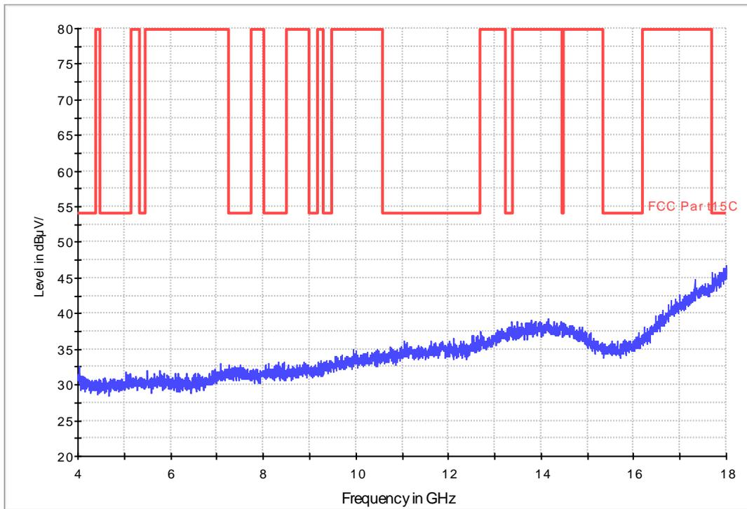
Fig. 35 Radiated Spurious Emission (802.11b, Ch6, 4 GHz-18 GHz)
