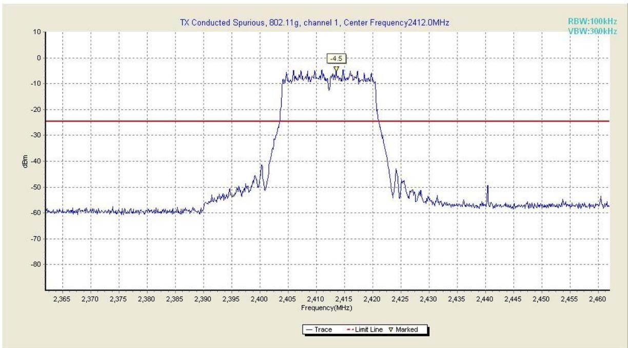
**Fig. 23 Conducted Spurious Emission (802.11g, Ch1, Center Frequency)**
