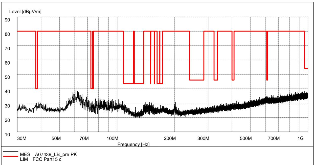
**Fig. 30 Radiated Spurious Emission (802.11b, Ch1, 30 MHz-1 GHz)**
