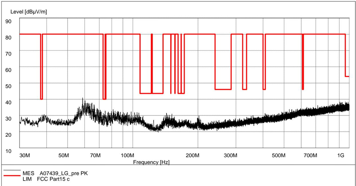
**Fig. 41 Radiated Spurious Emission (802.11g, Ch1, 30 MHz-1 GHz)**
