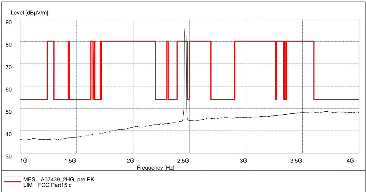
**Fig. 49 Radiated Spurious Emission (802.11g, Ch11, 1 GHz-4 GHz)**
