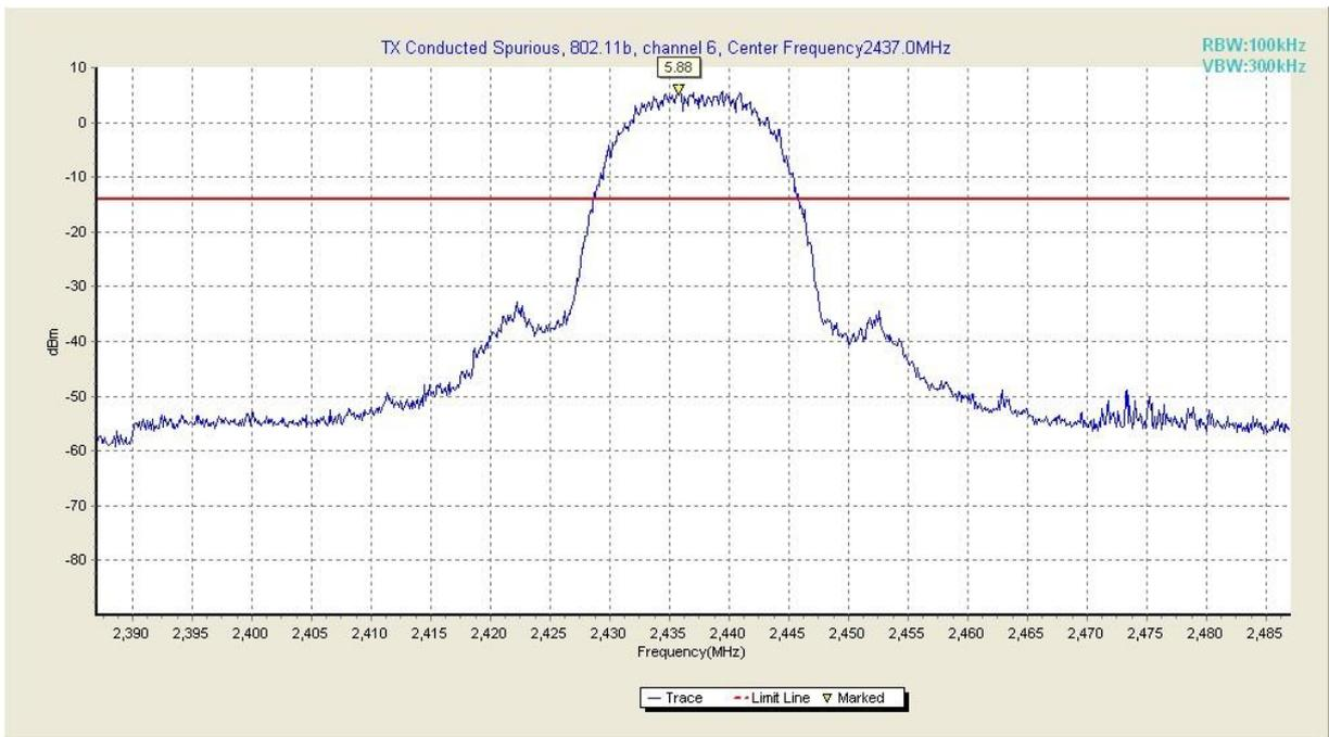
**Fig. 19 Conducted Spurious Emission (802.11b, Ch6, Center Frequency)**
