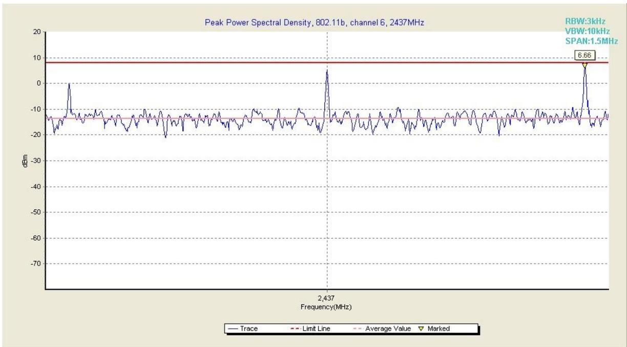
**Fig. 2 Power Spectral Density (802.11b, Ch 6)**
