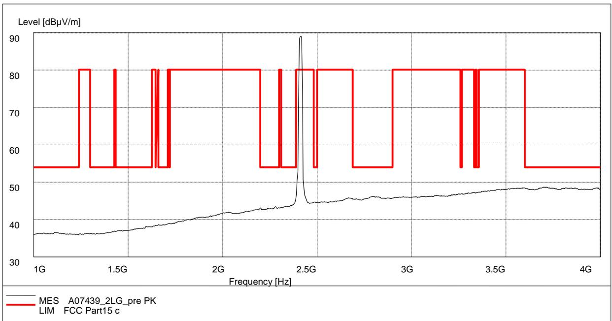
**Fig. 42 Radiated Spurious Emission (802.11g, Ch1, 1 GHz-4 GHz)**
