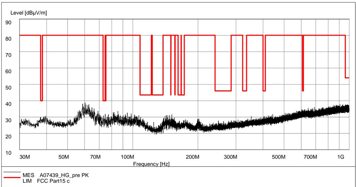
**Fig. 48 Radiated Spurious Emission (802.11g, Ch11, 30 MHz-1 GHz)**
