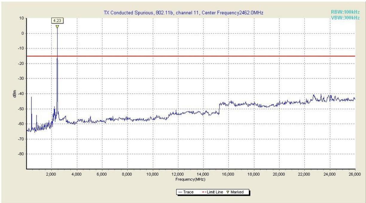
**Fig. 22 Conducted Spurious Emission (802.11b, Ch11, 30 MHz-26 GHz)**
