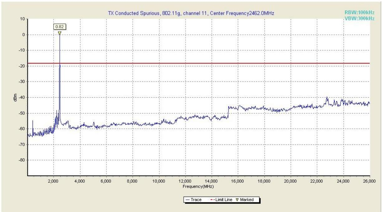
**Fig. 28 Conducted Spurious Emission (802.11g, Ch11, 30 MHz-26 GHz)**
