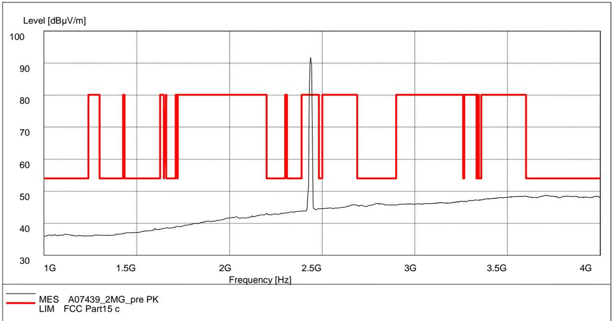
**Fig. 45 Radiated Spurious Emission (802.11g, Ch6, 1 GHz-4 GHz)**
