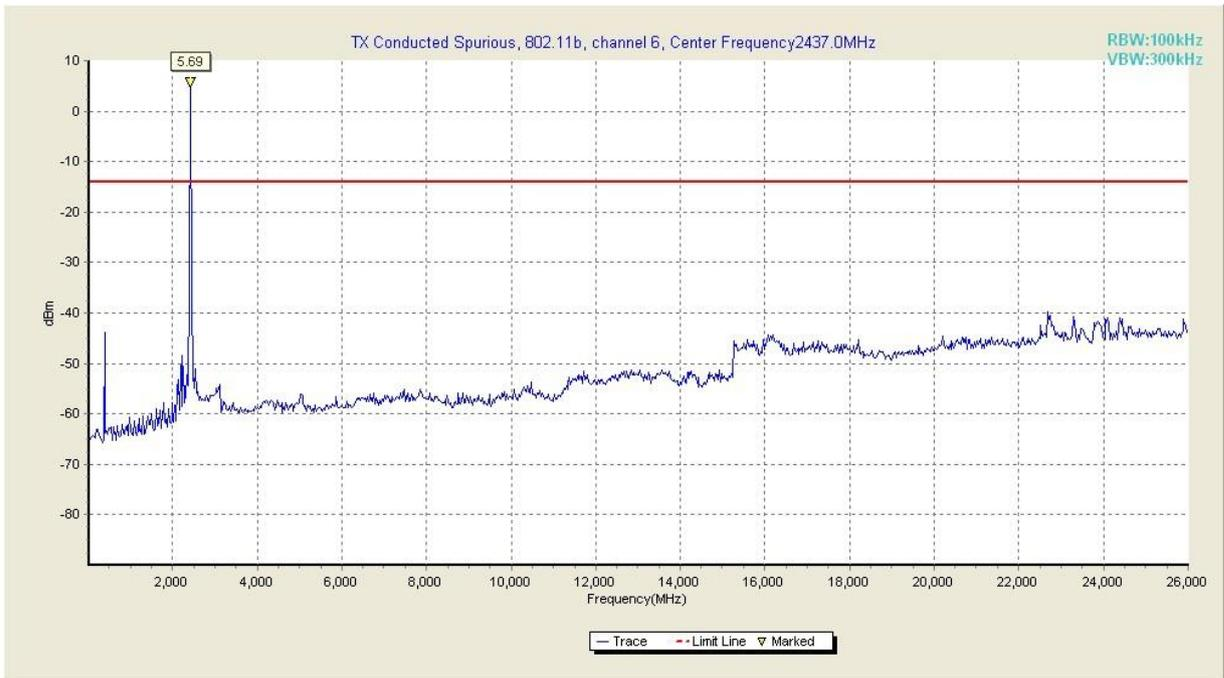
**Fig. 20 Conducted Spurious Emission (802.11b, Ch6, 30 MHz-26 GHz)**
