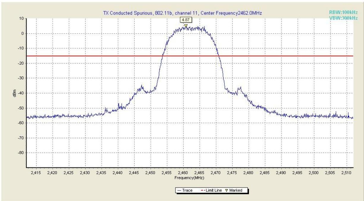
**Fig. 21 Conducted Spurious Emission (802.11b, Ch11, Center Frequency)**
