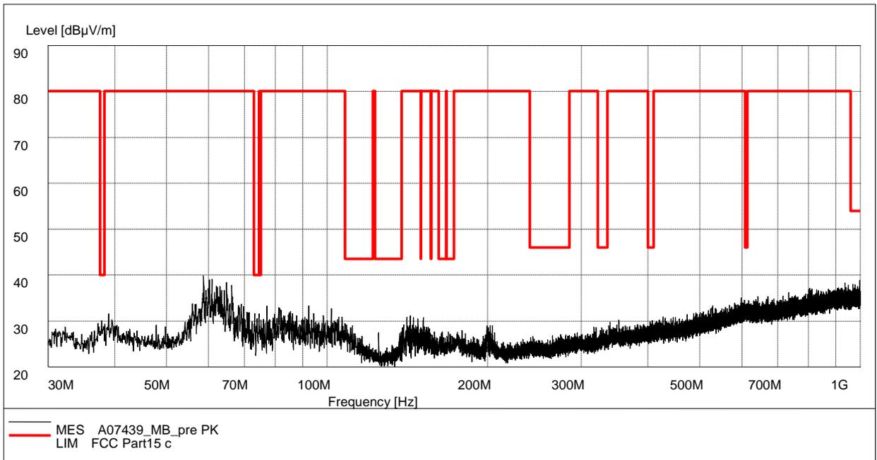
**Fig. 33 Radiated Spurious Emission (802.11b, Ch6, 30 MHz-1 GHz)**
