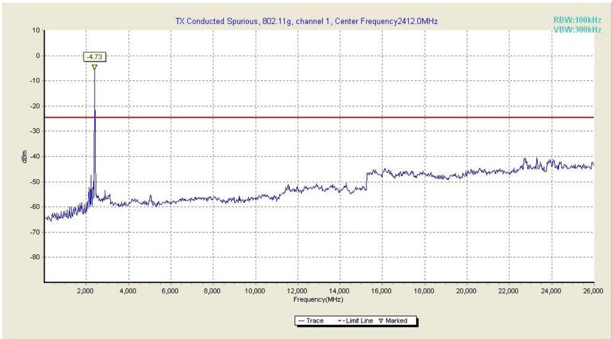
**Fig. 24 Conducted Spurious Emission (802.11g, Ch1, 30 MHz-26 GHz)**
