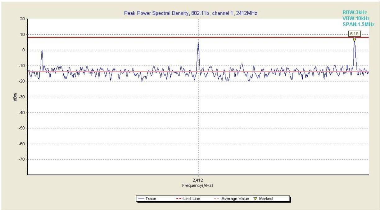
**Fig. 1 Power Spectral Density (802.11b, Ch 1)**
