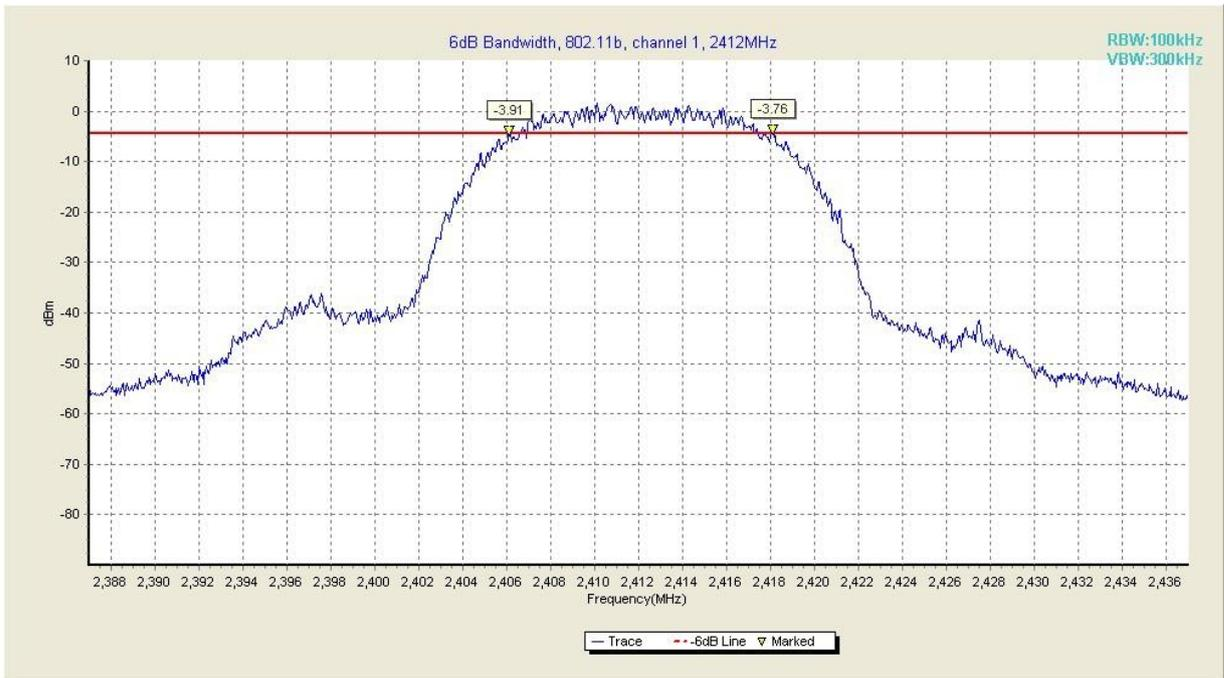
**Fig. 7 Occupied 6dB Bandwidth (802.11b, Ch 1)**
