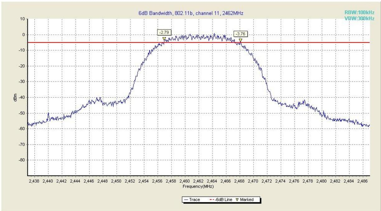
**Fig. 9 Occupied 6dB Bandwidth (802.11b, Ch 11)**
