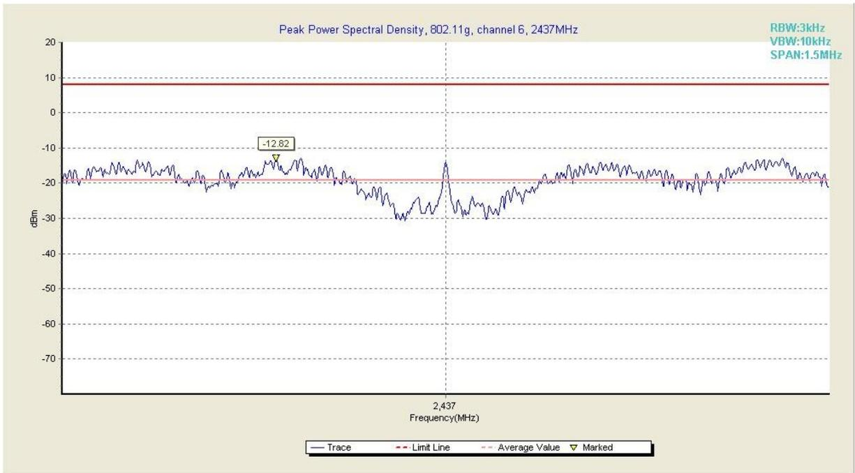
**Fig. 5 Power Spectral Density (802.11g, Ch 6)**
