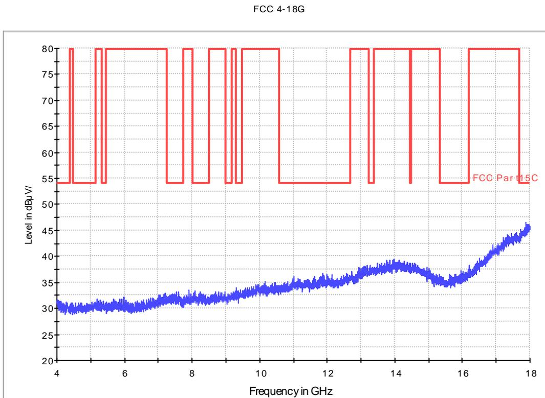
**Fig. 46 Radiated Spurious Emission (802.11g, Ch6, 4 GHz-18 GHz)**
