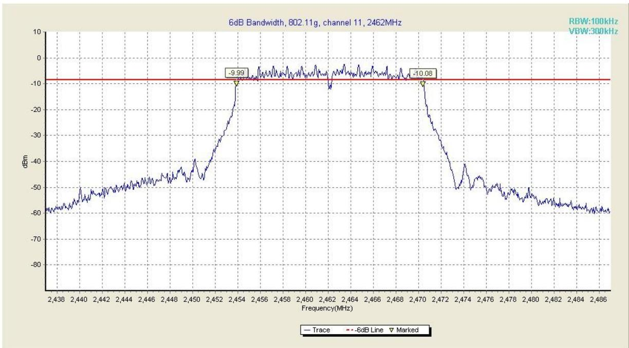
**Fig. 12 Occupied 6dB Bandwidth (802.11g, Ch 11)**
