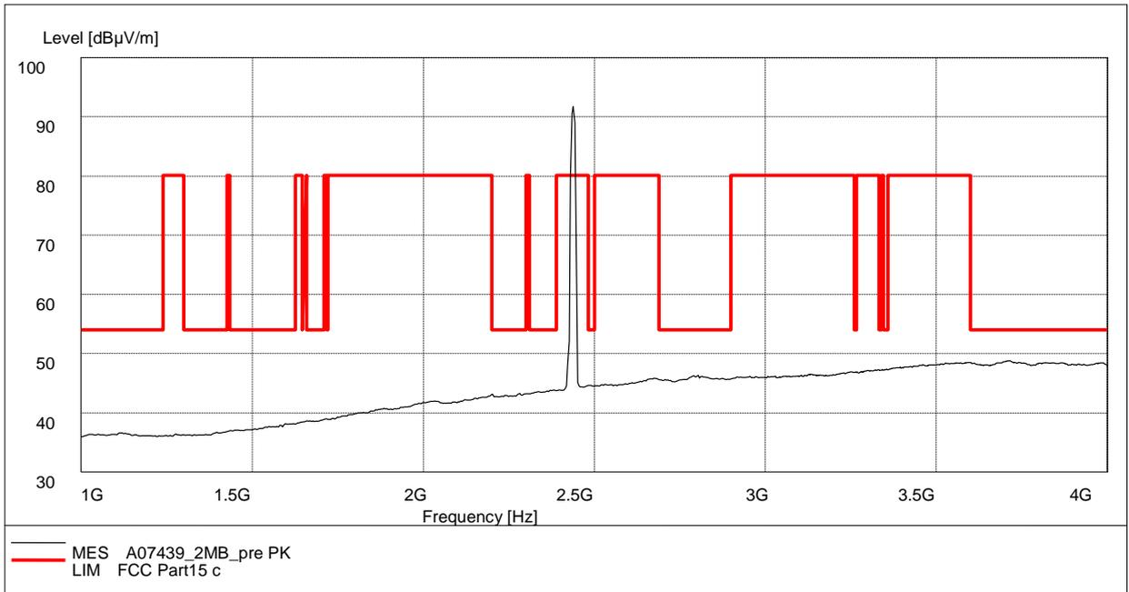
**Fig. 34 Radiated Spurious Emission (802.11b, Ch6, 1 GHz-4 GHz)**
