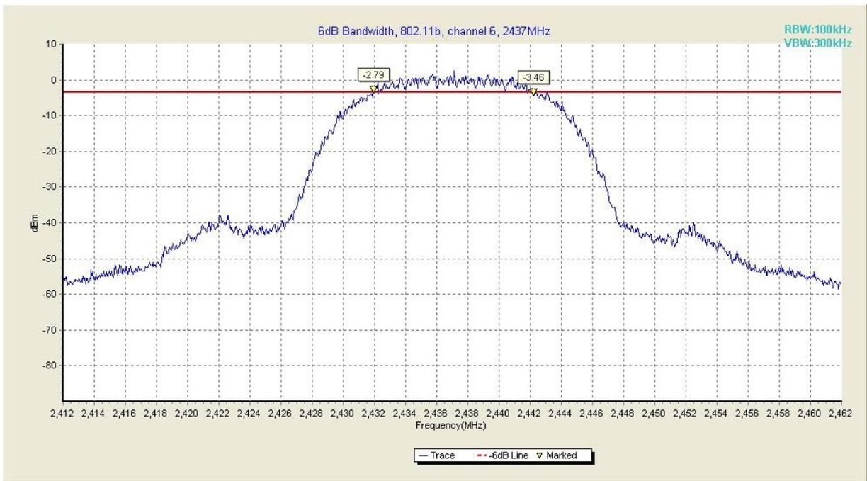
**Fig. 8 Occupied 6dB Bandwidth (802.11b, Ch 6)**
