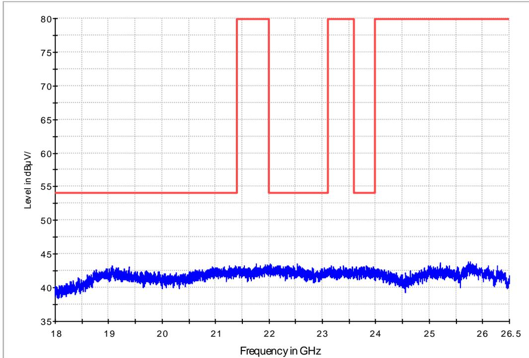
**Fig. 51 Radiated emission: 18 GHz - 26.5 GHz**
