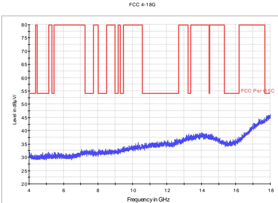
**Fig. 32 Radiated Spurious Emission (802.11b, Ch1, 4 GHz-18 GHz)**
