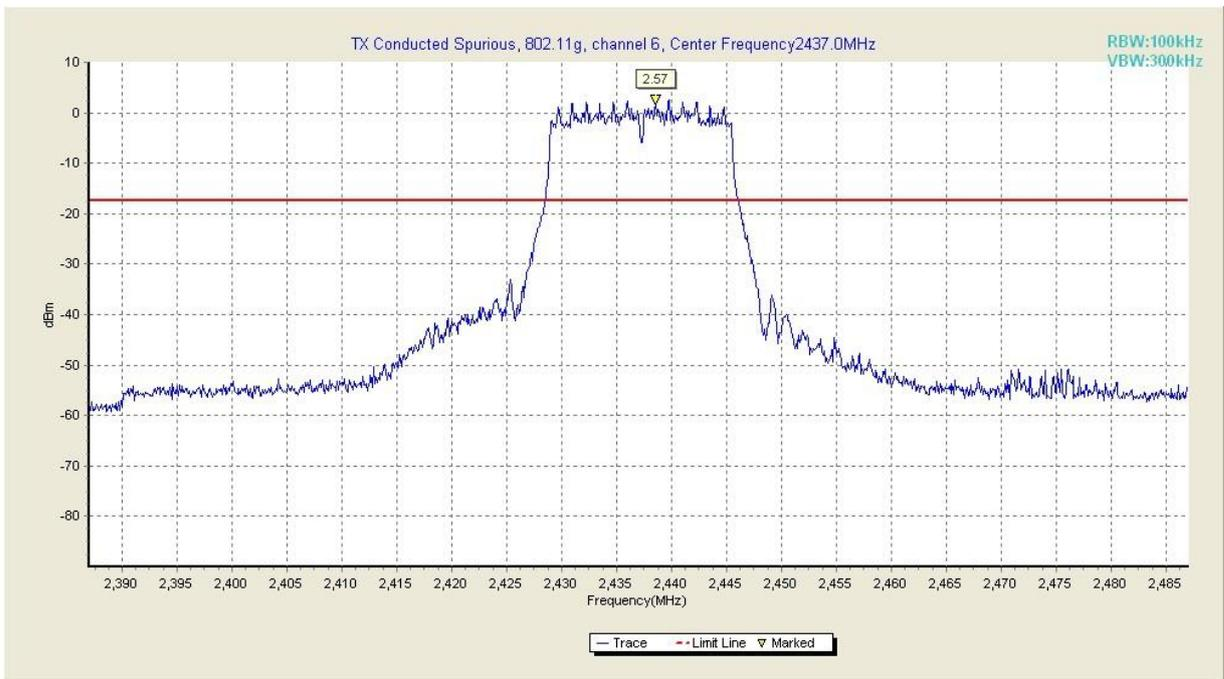
**Fig. 25 Conducted Spurious Emission (802.11g, Ch6, Center Frequency)**
