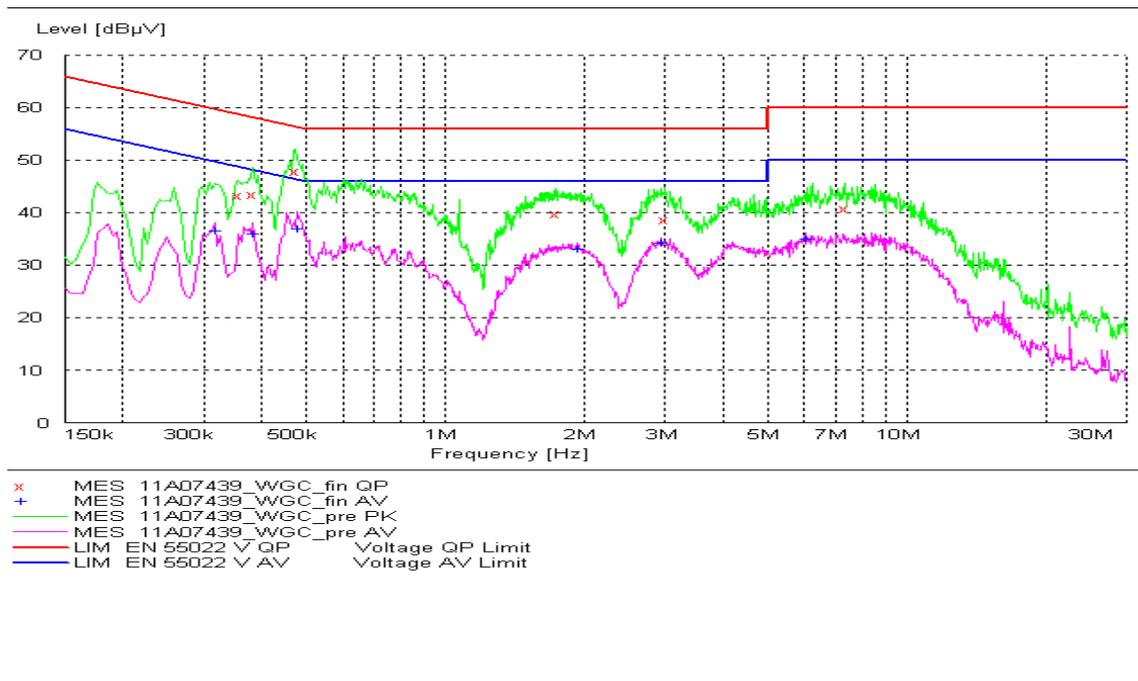
Fig. 52 AC Powerline Conducted Emission-802.11g-Transmitter
