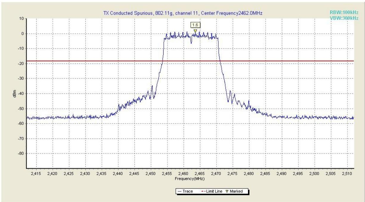
**Fig. 27 Conducted Spurious Emission (802.11g, Ch11, Center Frequency)**
