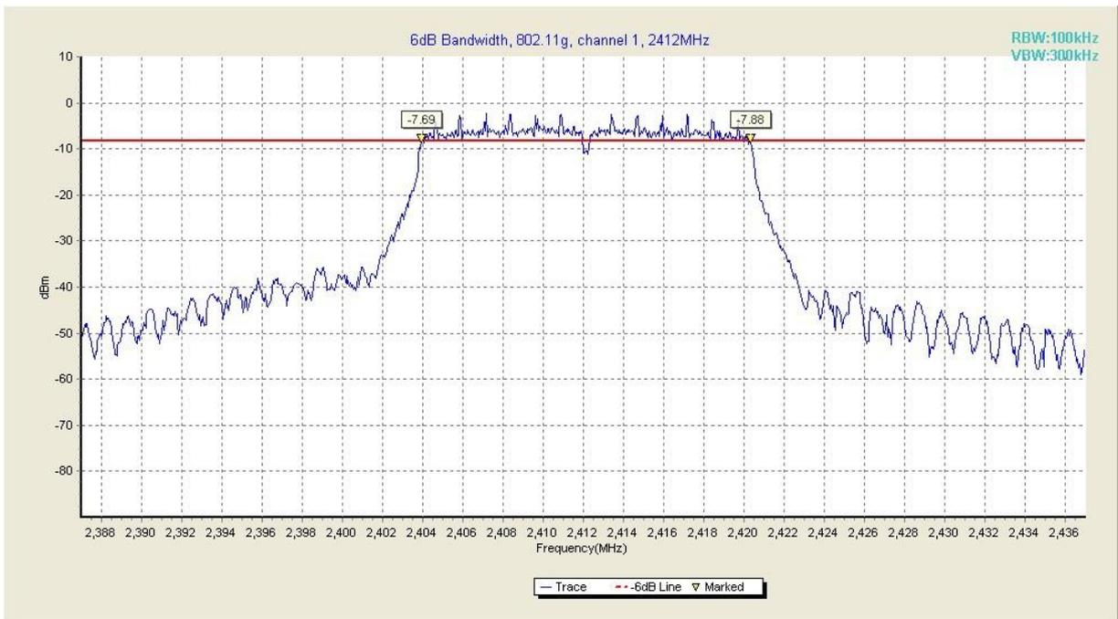
**Fig. 10 Occupied 6dB Bandwidth (802.11g, Ch 1)**
