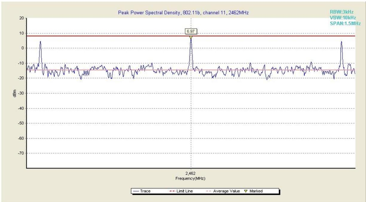
**Fig. 3 Power Spectral Density (802.11b, Ch 11)**
