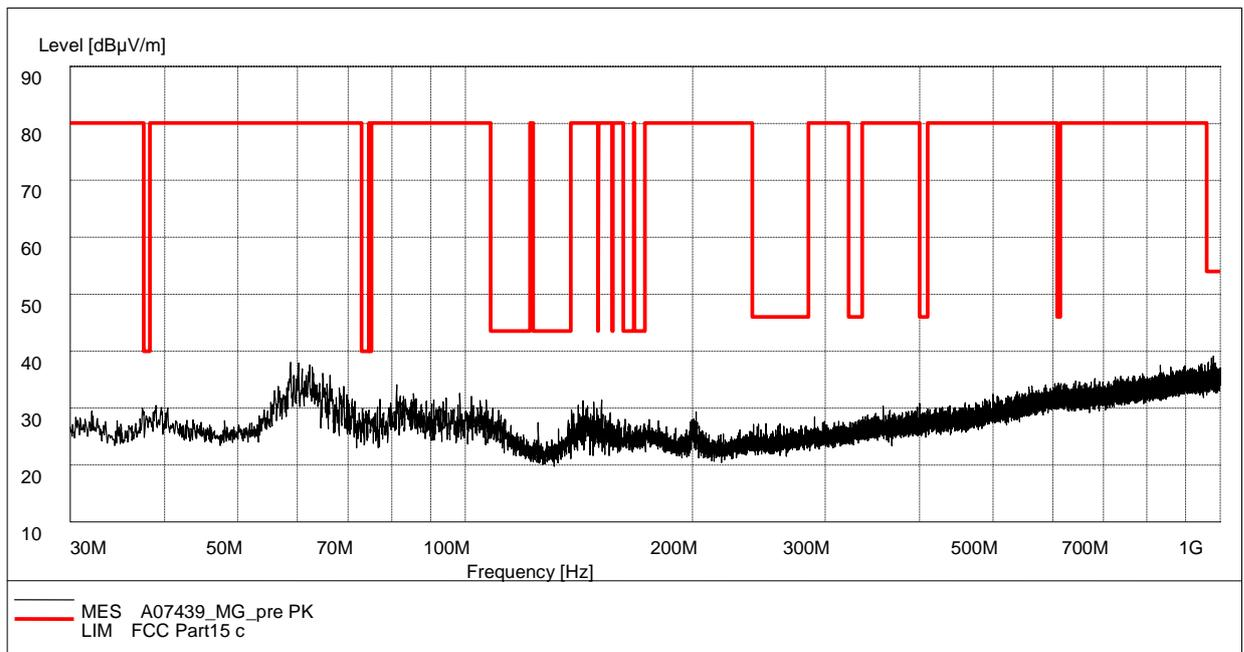
Fig. 44 Radiated Spurious Emission (802.11g, Ch6, 30 MHz-1 GHz)
