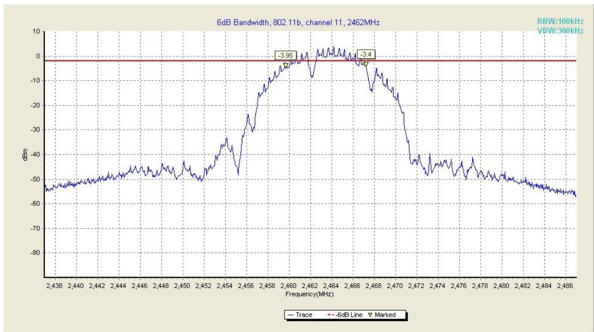
Fig. 9 Occupied 6dB Bandwidth (802.11b, Ch 11)
