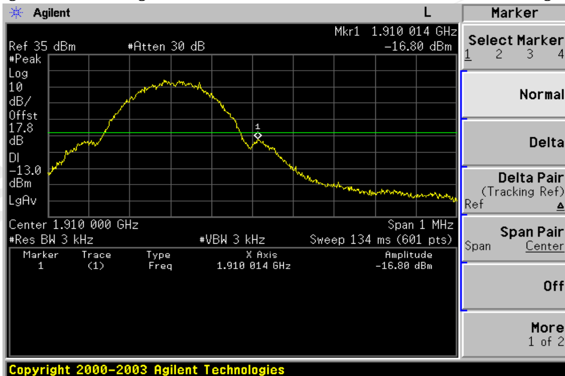
Figure 8-20: Band edge emission at antenna terminals –EGPRS 1900 Channel Highest
