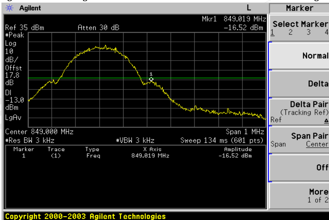
Figure 8-15: Band edge emission at antenna terminals –EGPRS 850 Channel Highest
