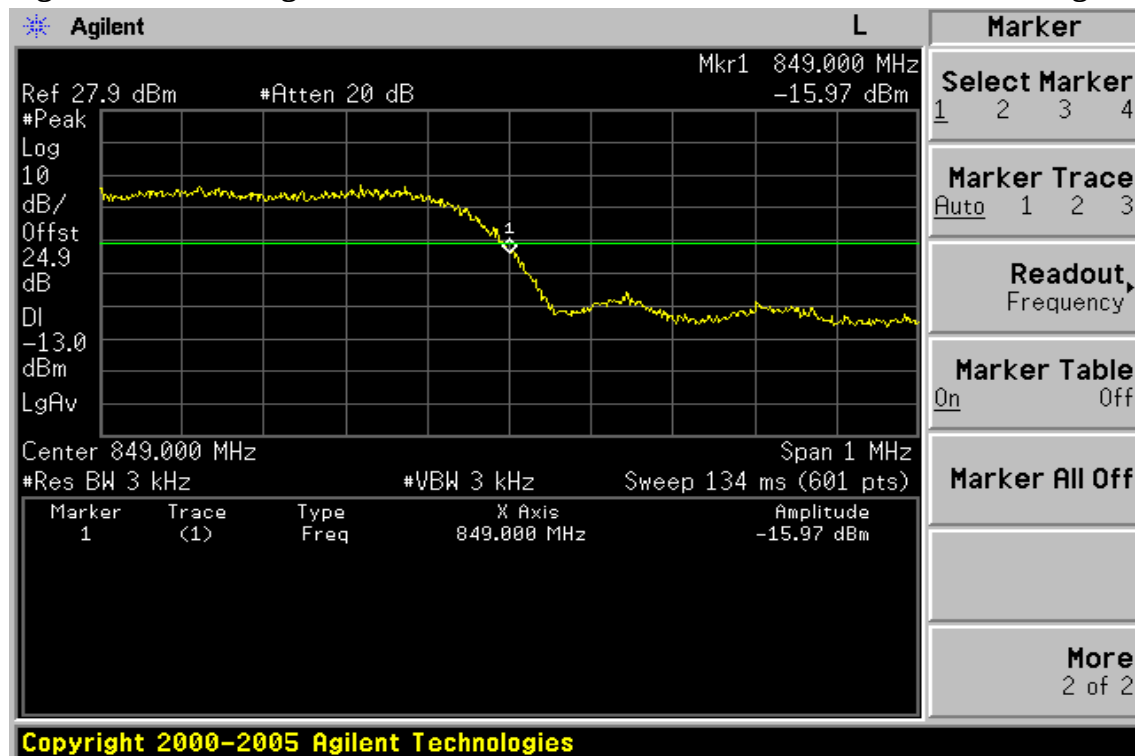
Figure 8-5: Band edge emission at antenna terminals – CDMA850 Channel Highest
