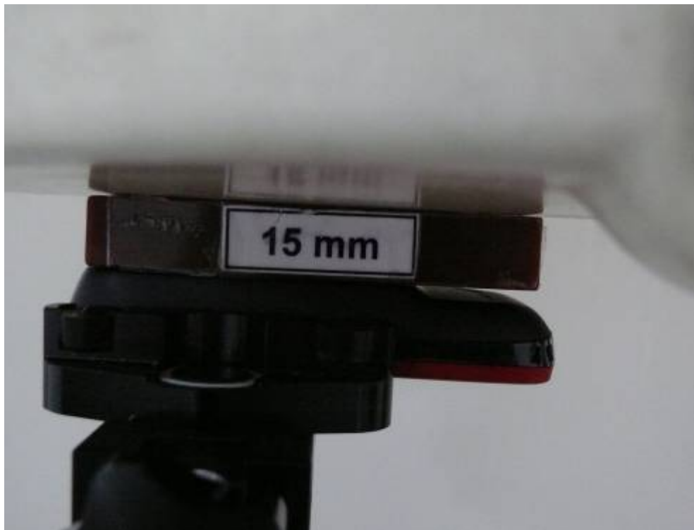
Picture 11: Body, The EUT display towards ground, the distance from handset to the bottom of the Phantom is 15mm (The spacer was removed during testing)
