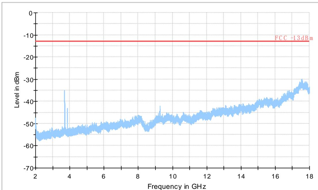
**A.2.3.5 RADIATED SPURIOUS EMISSIONS-Channel 9400: 2GHz – 18GHz**
