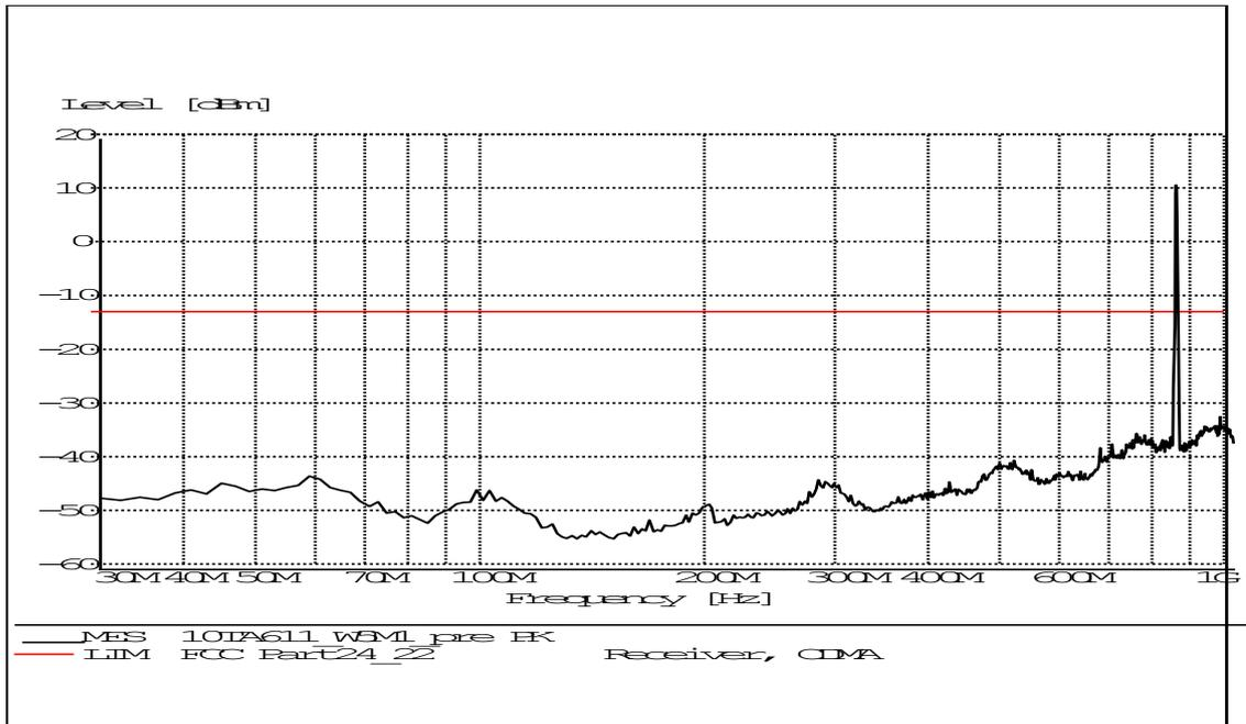
**A.2.3.13 RADIATED SPURIOUS EMISSIONS-Channel 4233: 30MHz – 1GHz**
