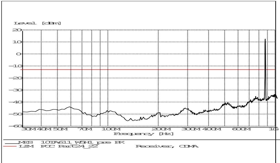
**A.2.3.14 RADIATED SPURIOUS EMISSIONS-Channel 4132: 1GHz – 10GHz**
