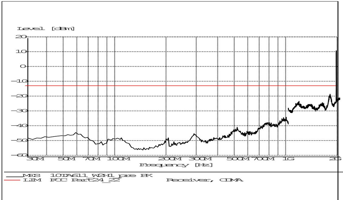
**A.2.3.4 RADIATED SPURIOUS EMISSIONS-Channel 9262: 2GHz – 18GHz**
