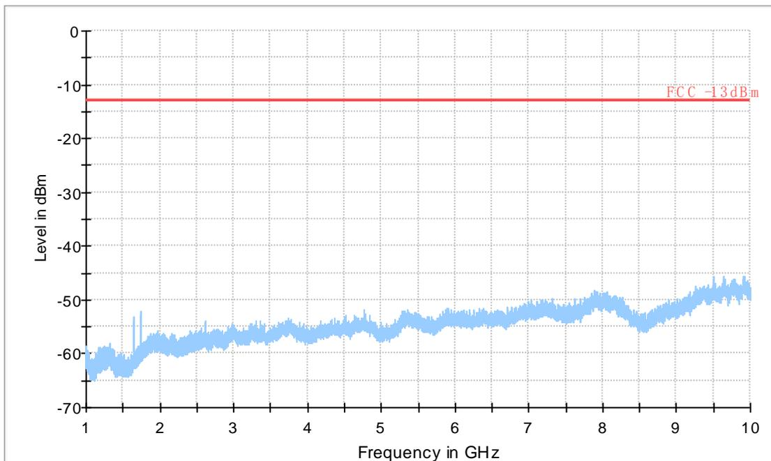
**A.2.3.15 RADIATED SPURIOUS EMISSIONS-Channel 4183: 1GHz – 10GHz**
