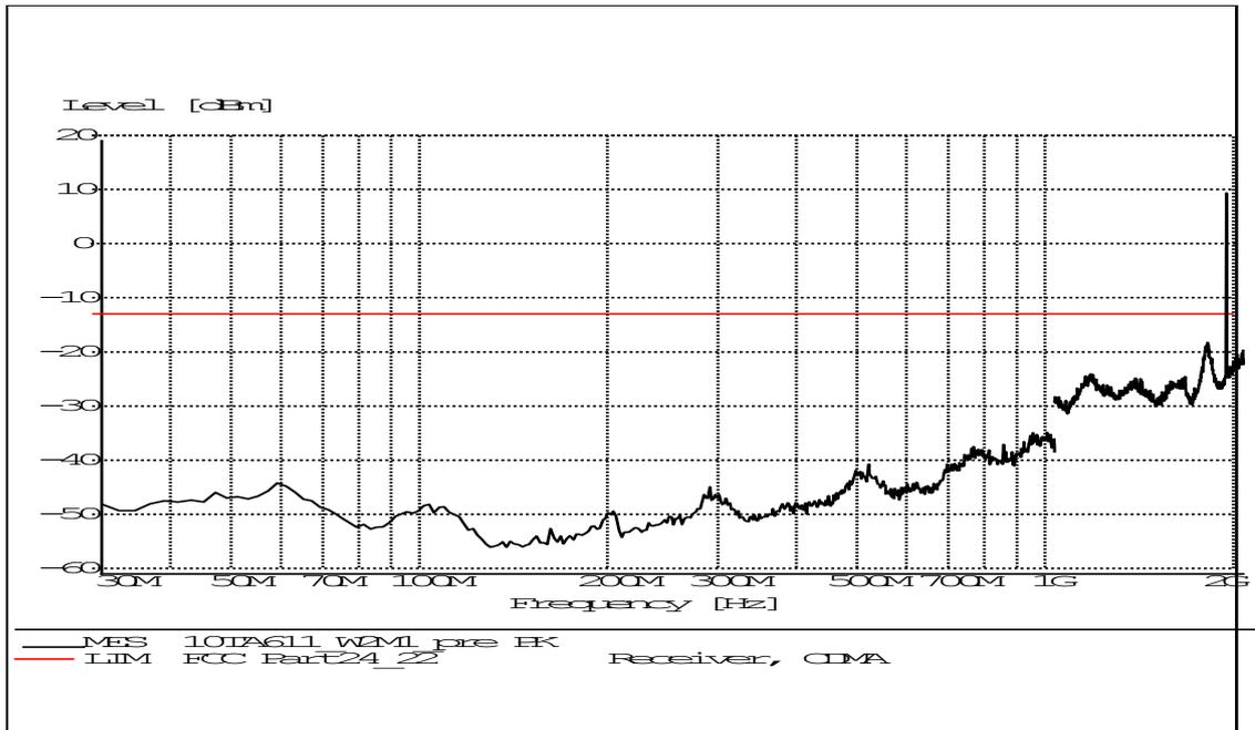
**A.2.3.3 RADIATED SPURIOUS EMISSIONS-Channel 9538: 30MHz – 2GHz**
