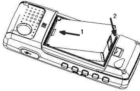
Close the case by locating the top of the plastic cover into the grooves and gently pushing the cover down to close it.
