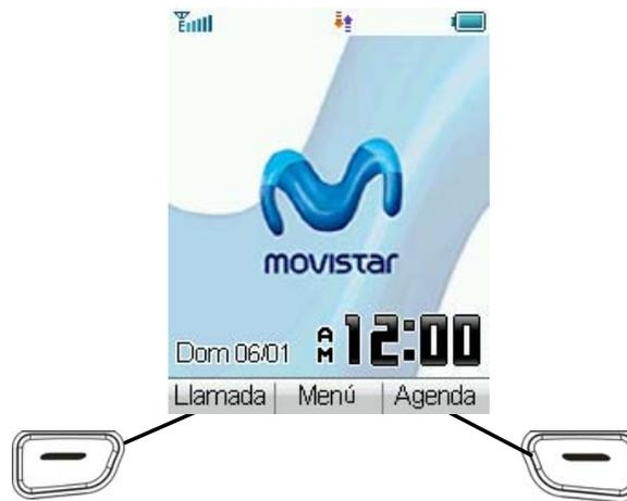
The left and right **Select Keys** are used to choose the options from the bottom of the screen.
