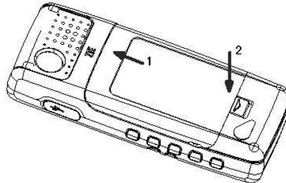
Make sure the latch closes properly. The rubber seal provides a tight fit so sometimes it is necessary
