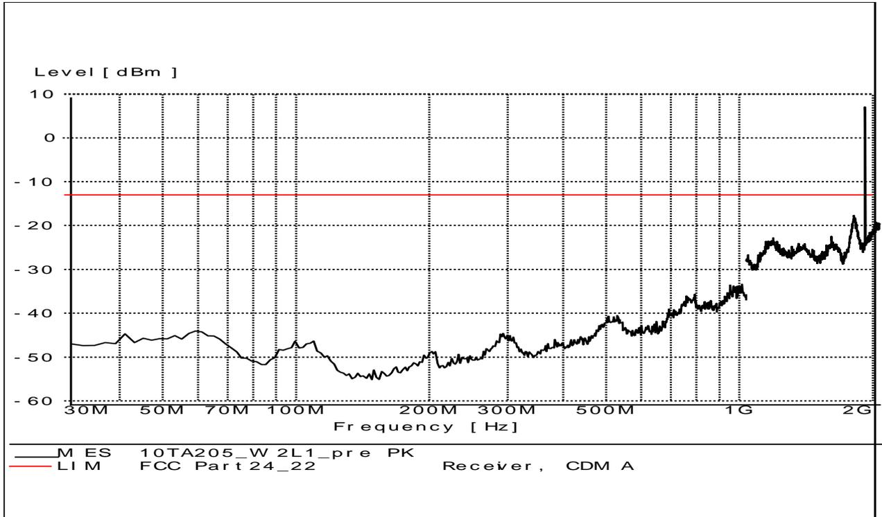
**A.2.3.2 RADIATED SPURIOUS EMISSIONS-Channel 9400: 30MHz – 2GHz**
