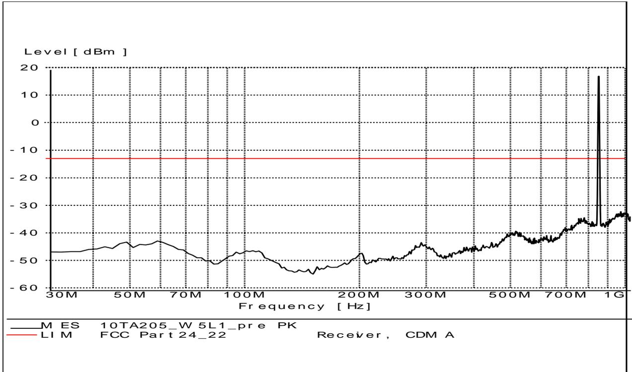
A.2.3.12 RADIATED SPURIOUS EMISSIONS-Channel 4183: 30MHz – 1GHz
