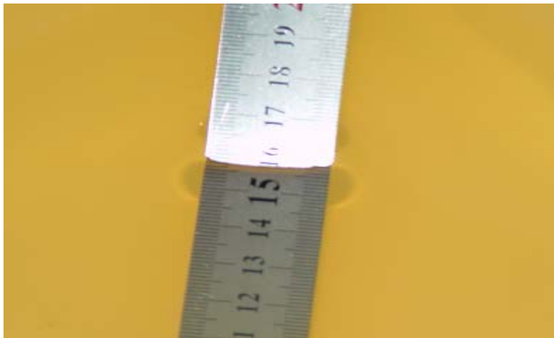
Liquid depth for SAR Measurement
