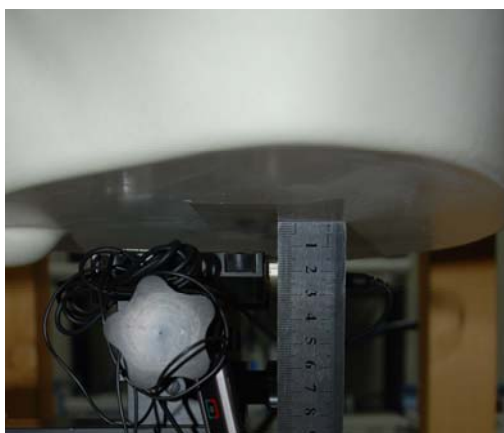
Fig 3 – Face away the phantom with the distance of 15mm
