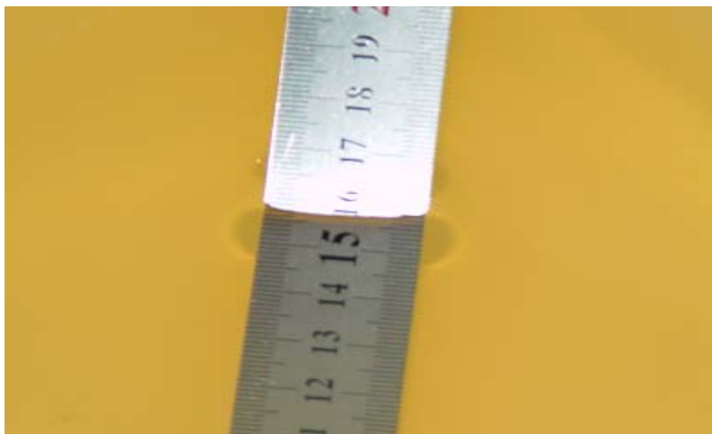
Liquid depth for SAR Measurement
