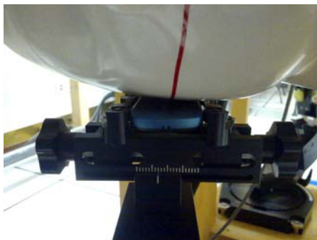
Fig 2 - Definition of the reference lines and points, on the phone and on the phantom and initial position
