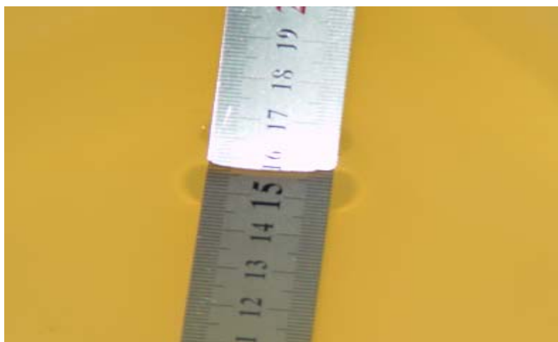
Liquid depth for SAR Measurement
