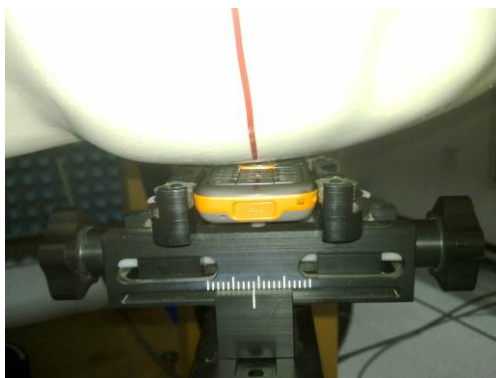
Definition of the reference lines and points, on the phone and on the phantom and initial position
