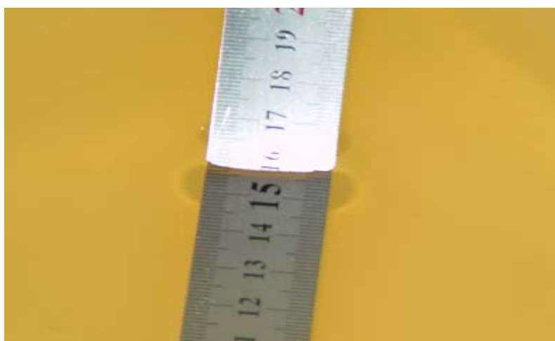
Liquid depth for SAR Measurement
