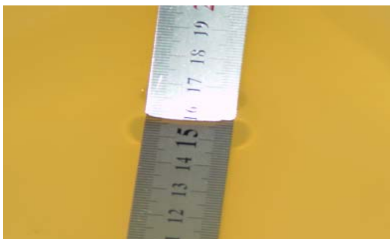
Liquid depth for SAR Measurement
