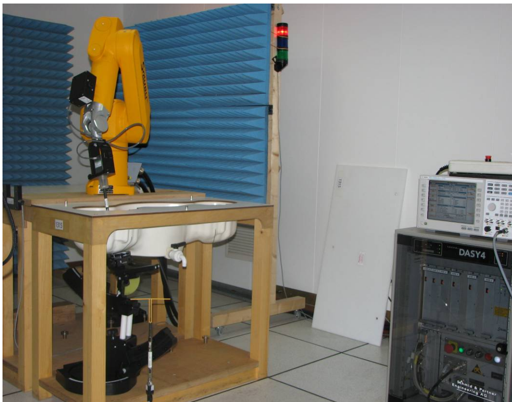
The measurement set-up with two SAM phantoms containing tissue simulating liquid
