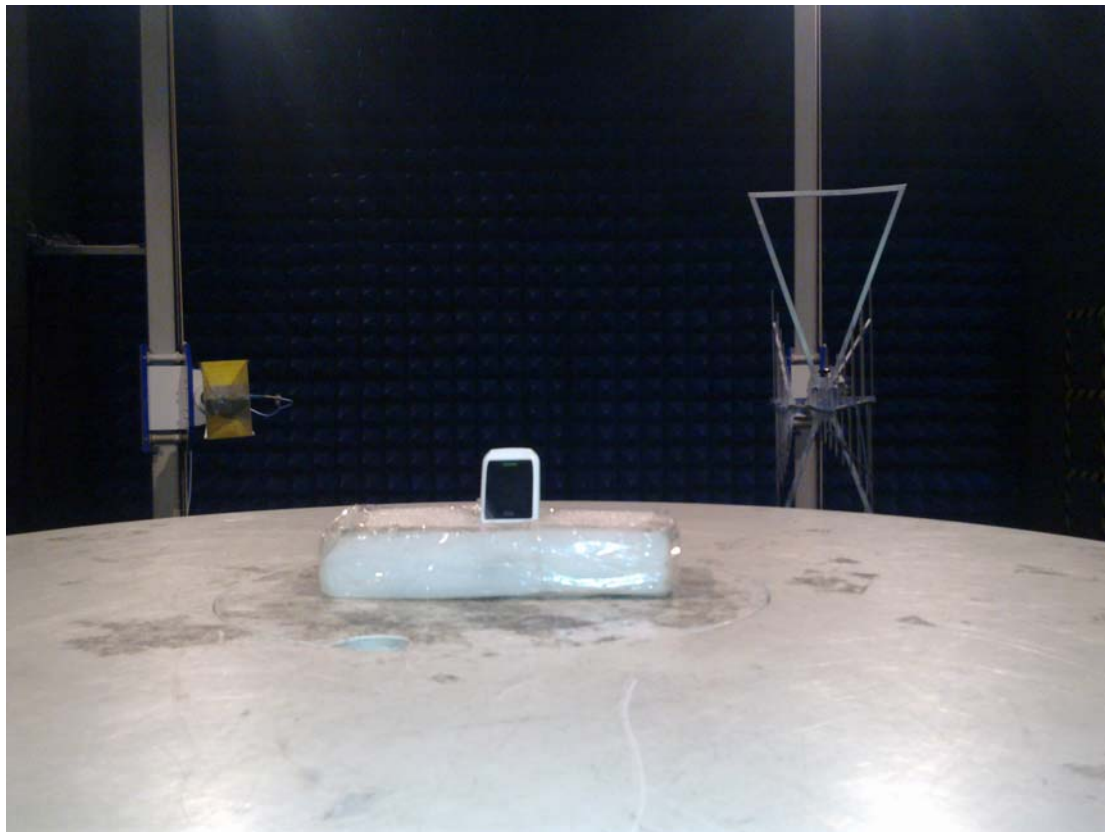
Radiated Spurious Emissions Test setup
