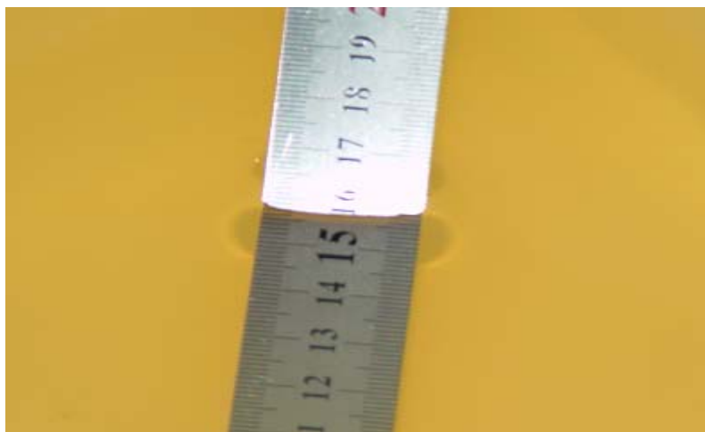
Liquid depth for SAR Measurement
