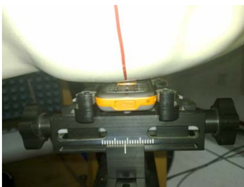
Fig 2 - Definition of the reference lines and points, on the phone and on the phantom and initial position
