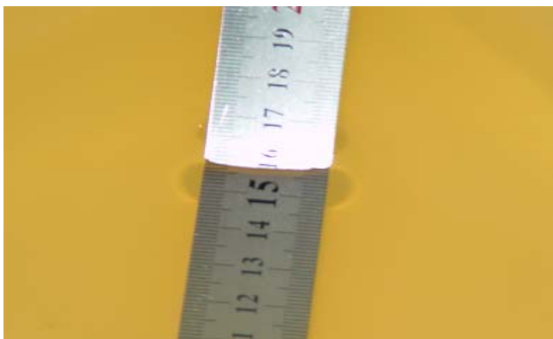
Liquid depth for SAR Measurement
