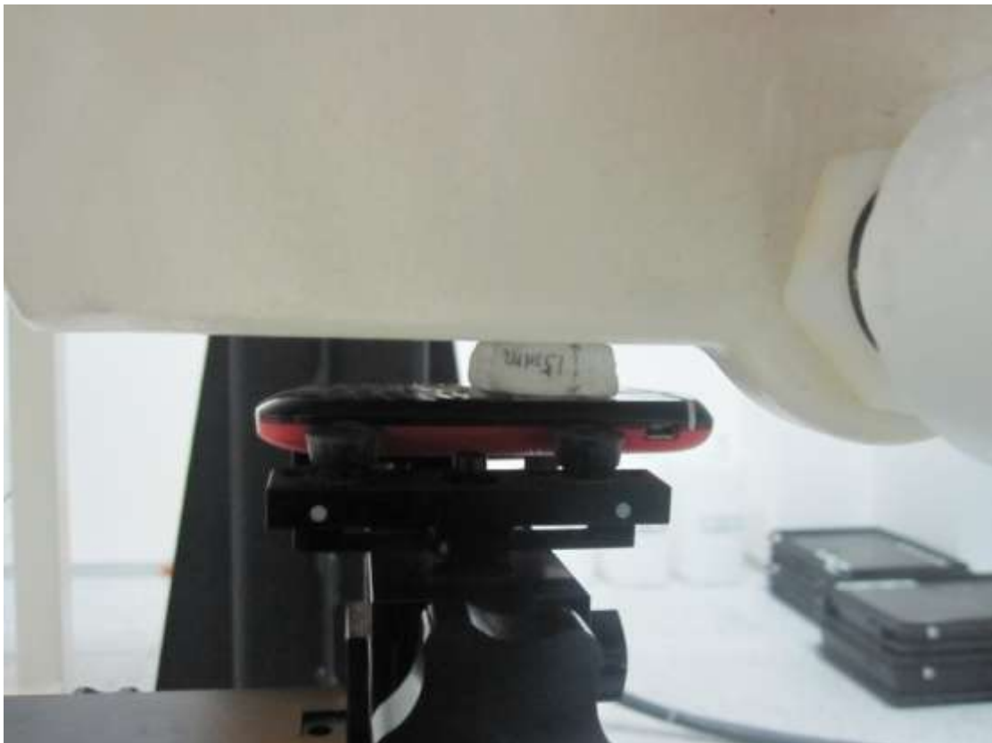
POSITION OF BODY TOWARDS PHANTOM WITH 15mm DISTANCE
