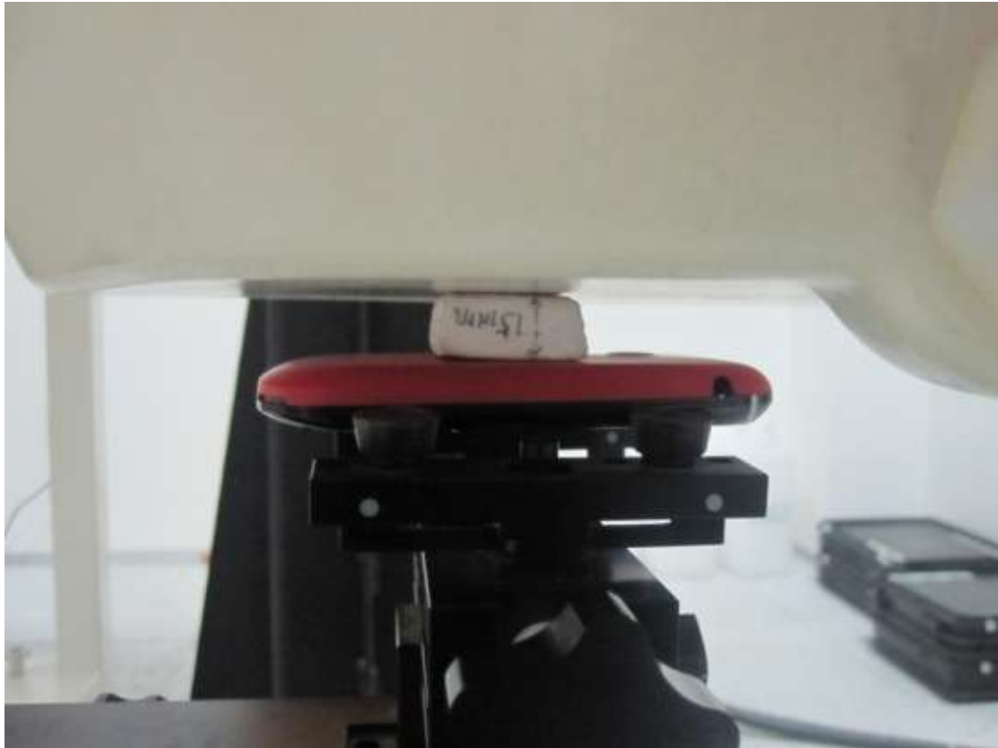
POSITION OF BODY TOWARDS GROUND WITH 15mm DISTANCE
