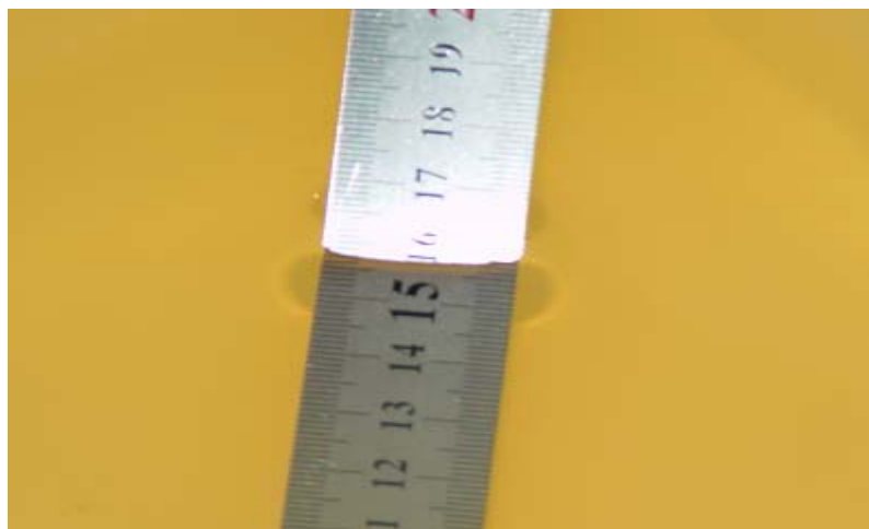
Liquid depth for SAR Measurement
