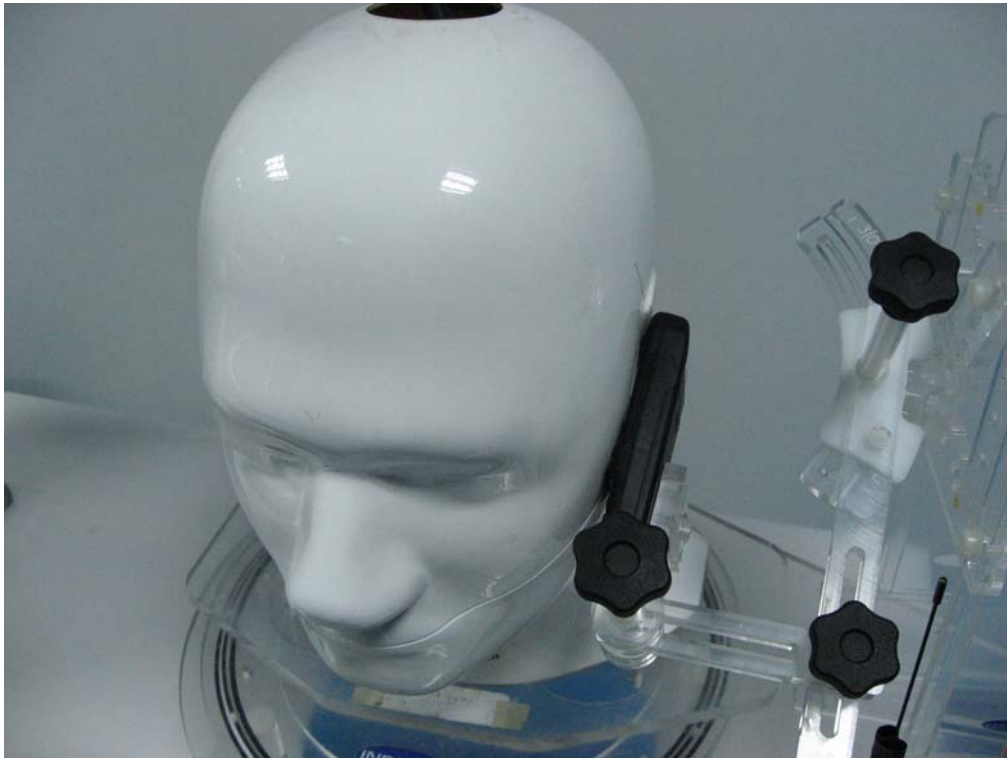
Fig.3 EUT Left Head Touch Cheek Position
