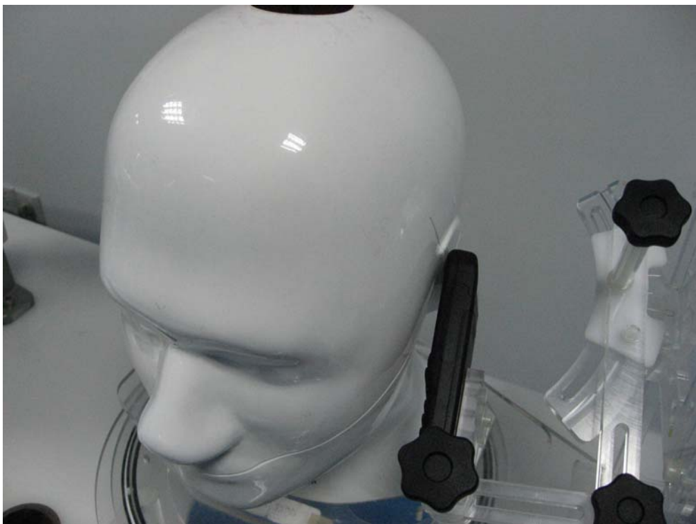
Fig.4 EUT Left Head Tilt15 Position
