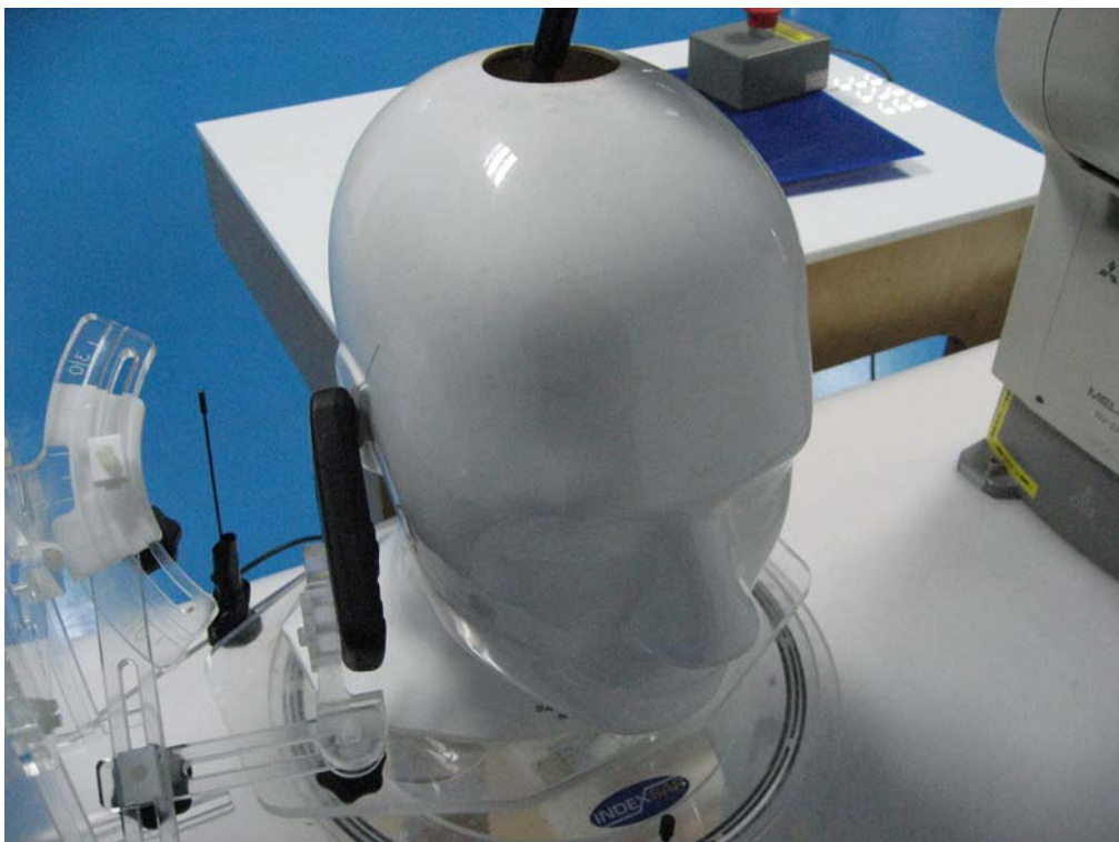
Fig.6 EUT Right Head Tilt15 Position
