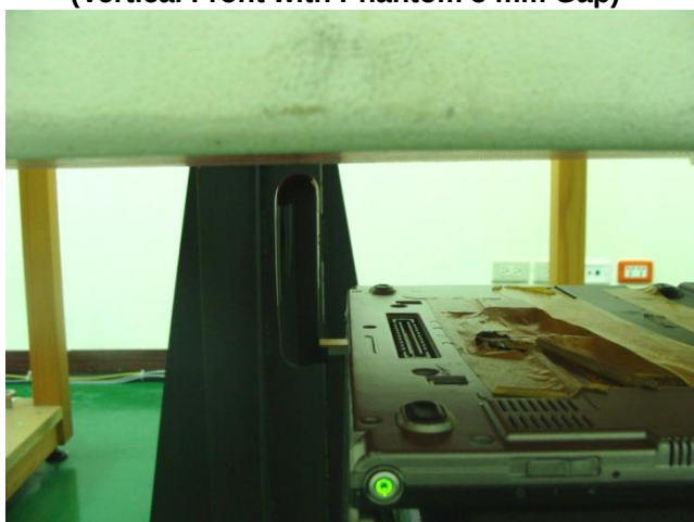
Direct Laptop Plug-in for Tip Mode (Tip Mode of the DUT with Phantom 5 mm Gap)
