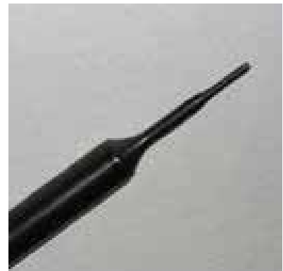
Figure 2. EX3DV4 E-field Probe
