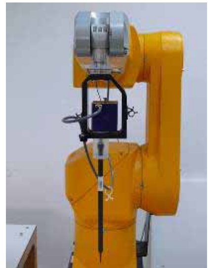
Figure 3. EX3DV4 E-field probe
