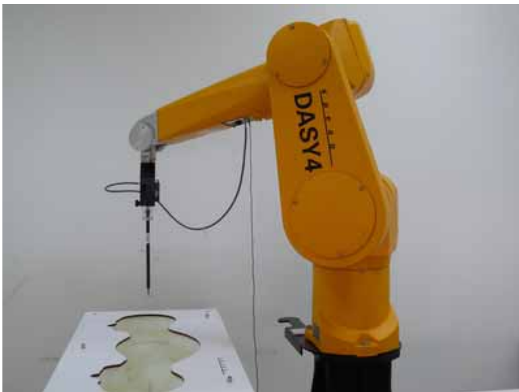
Picture 1: Specific Absorption Rate Test Layout
