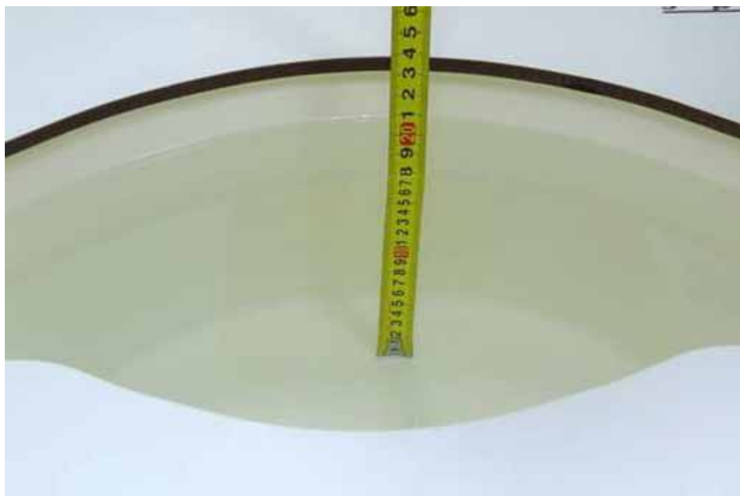
Picture 4: Liquid depth in the flat Phantom (1900 MHz)
