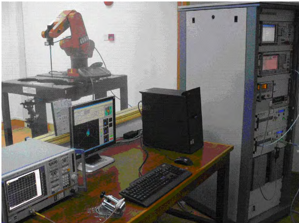
Figure B.1 COMOSAR Test Bench Test Layout
