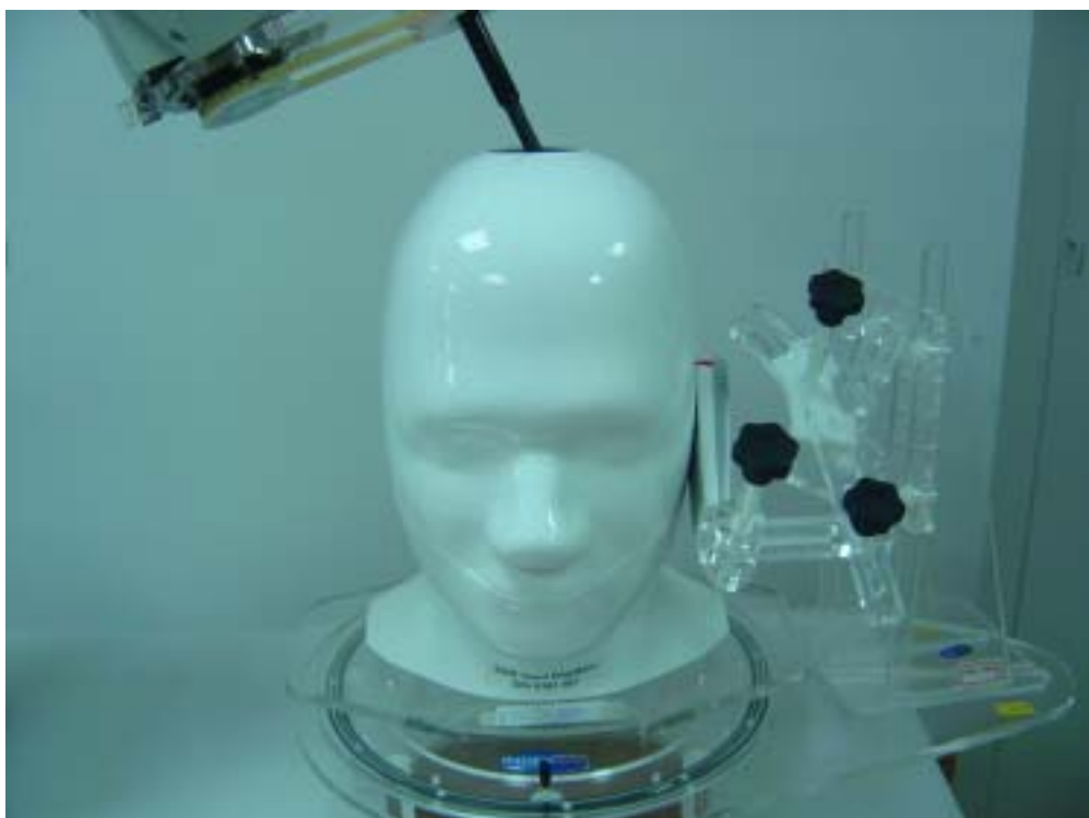
Fig.3 EUT Left Head Touch Cheek Position
