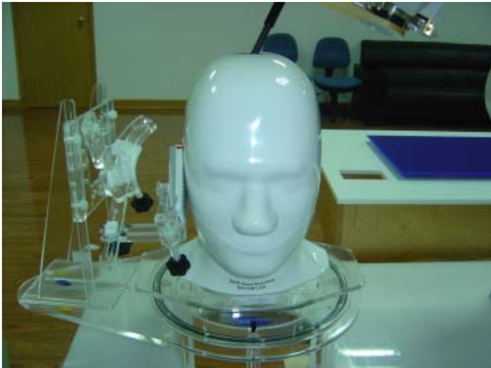
Fig.5 EUT Right Head Touch Cheek Position
