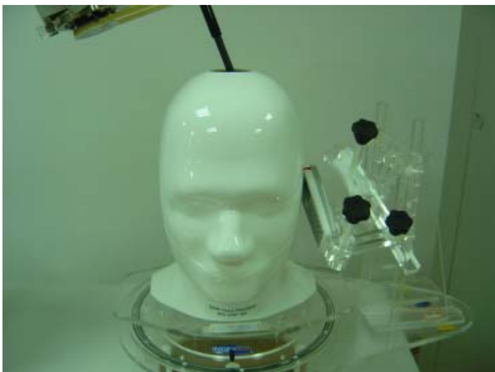
Fig.4 EUT Left Head Tilt15 Position
