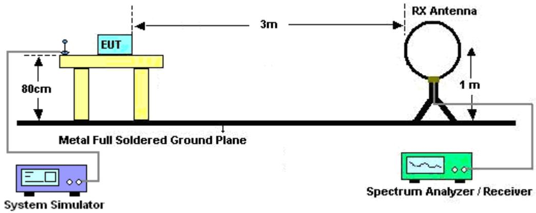
For radiated emissions from 30MHz to 1GHz
