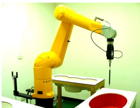
Fig 5.5 Photo of DASY5
