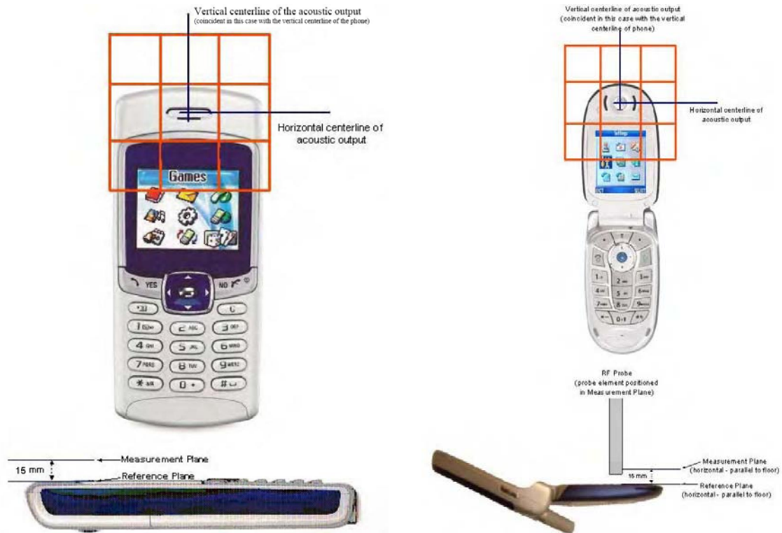
Fig 9.1 A typical EUT reference and plane for HAC measurements
