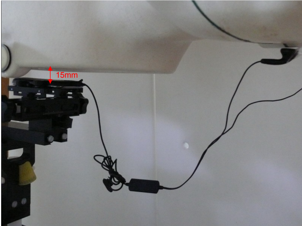
Picture 13: Body with earphone, The EUT display towards ground, the distance from handset to the bottom of the Phantom is 15mm
