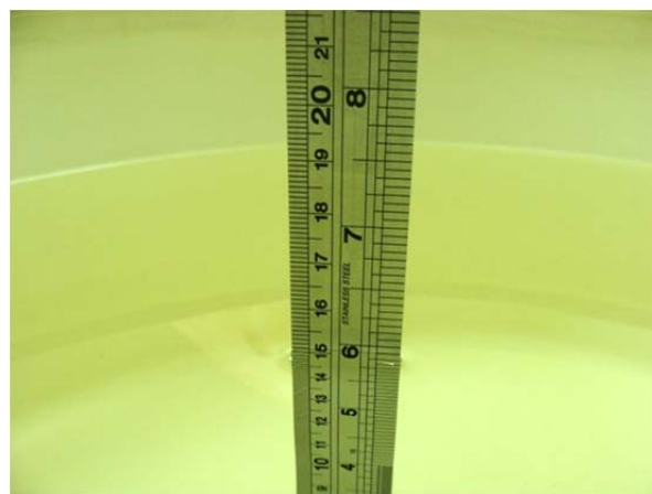
Fig 6.2 Photo of Liquid Height for Body SAR
