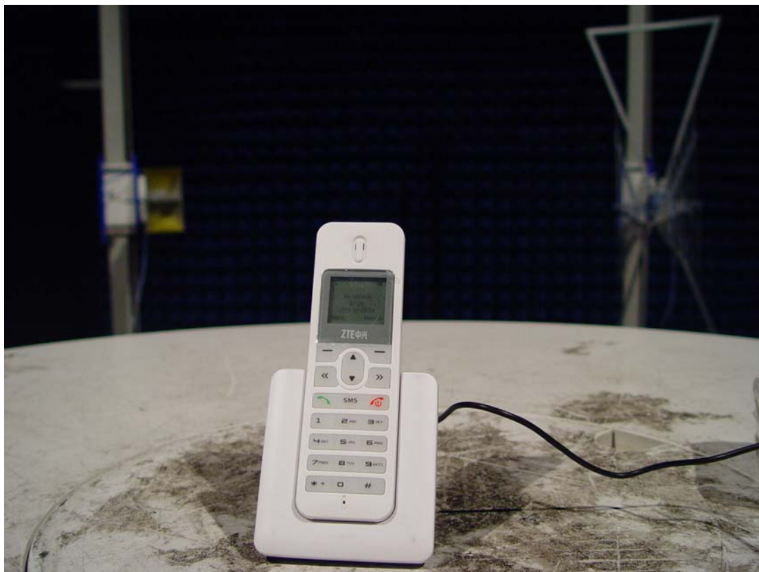
Radiated Spurious Emissions Test setup
