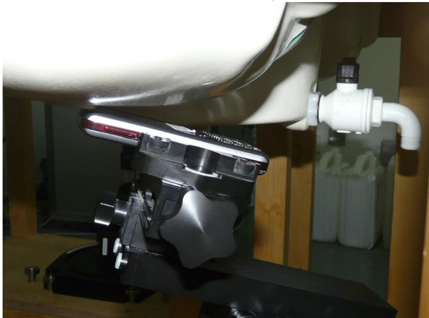
Picture 5 Head SAR tilt position
