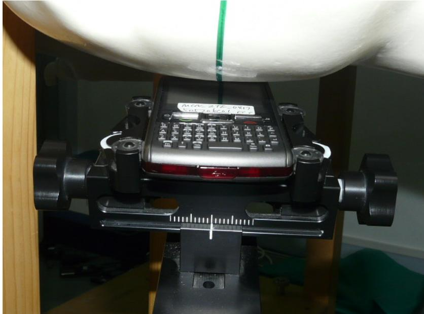
Picture 4 Head SAR tilt position
