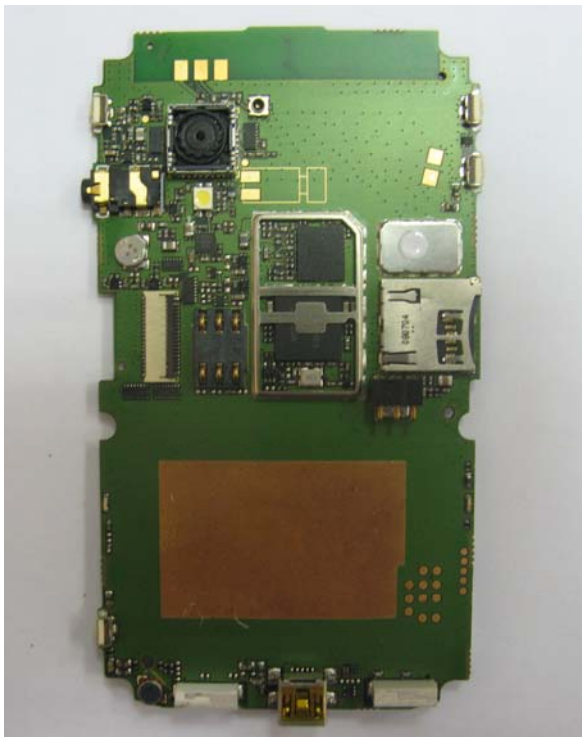
Picture 4: The top view of the PCB with the shielding cover removed
