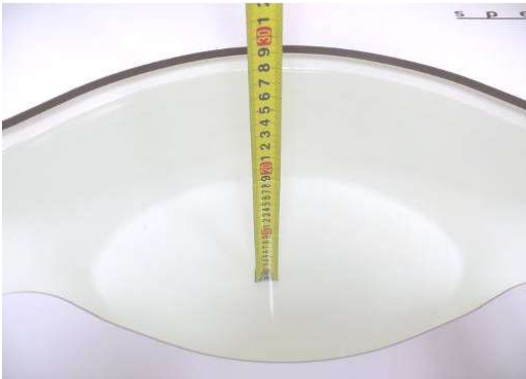
Picture D.6: Liquid depth in the flat Phantom (2450 MHz) (18.6cm deep)
