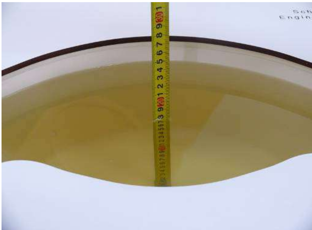
Picture D.2: Liquid depth in the flat Phantom (835MHz) (17.5cm deep)
