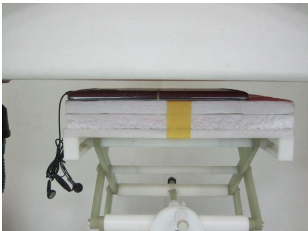
Bottom Face of the EUT with Phantom 1.4 cm Gap
