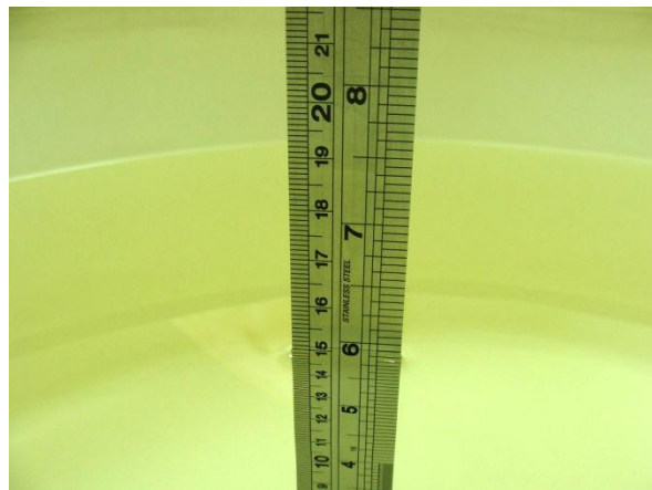
Fig 6.2 Photo of Liquid Height for Body SAR
