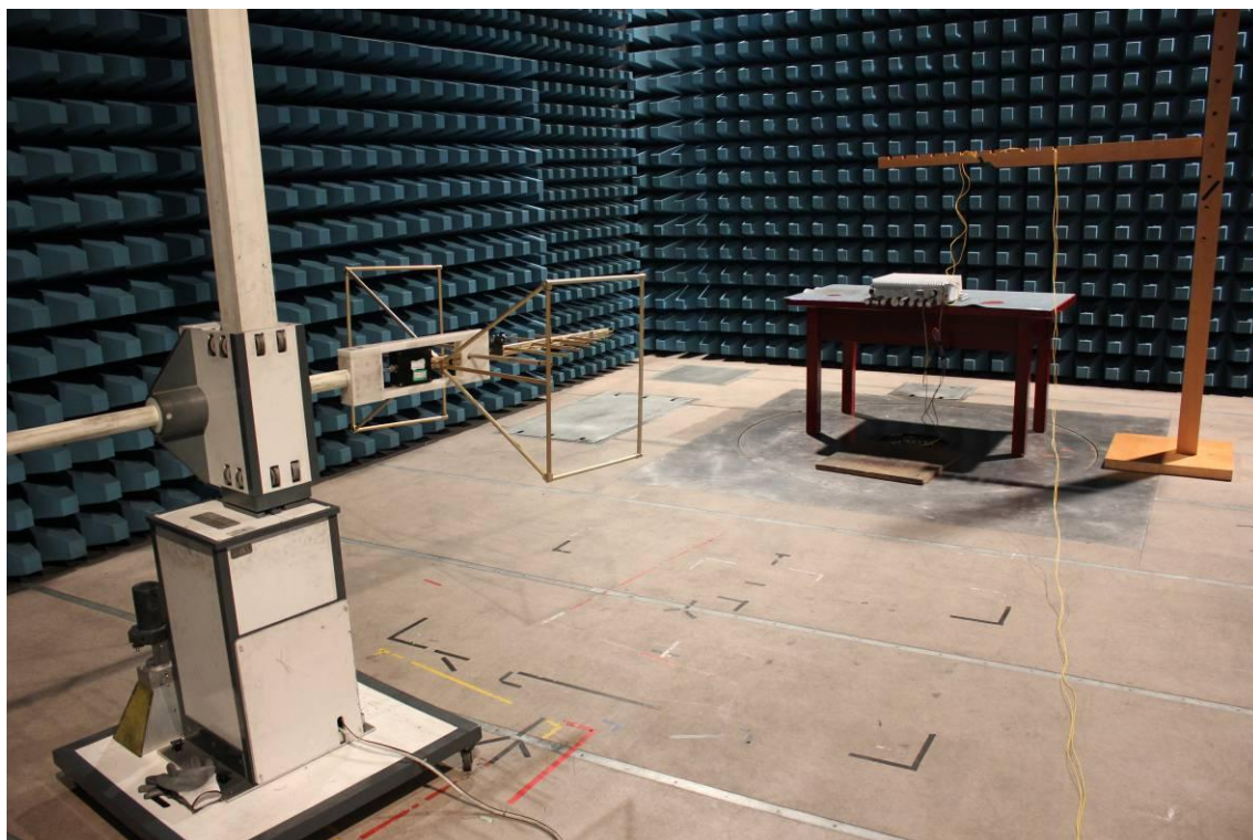
Fig.1 Radiated Spurious Emissions test (below 3 GHz) (DC)
