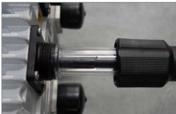
Figure 4-45 Insert Transparent Sleeve
