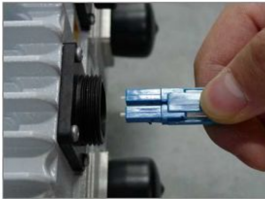
Figure 4-44 Insert Optical Fiber
